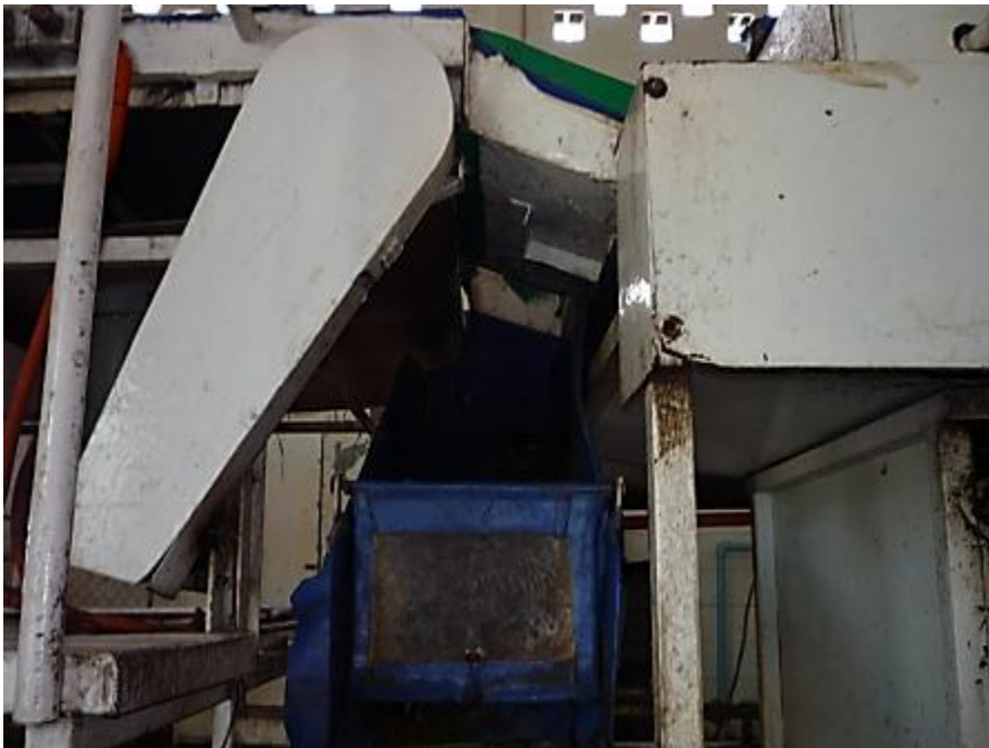
Figure 6-8 Fruit selector in a packinghouse in Escuinapa, Sinaloa, Mexico The device is installed before the fruit sorter (Figure 6-7, above). Large mangos that are ineligible for HWT drop into the container. (Photo by author)
