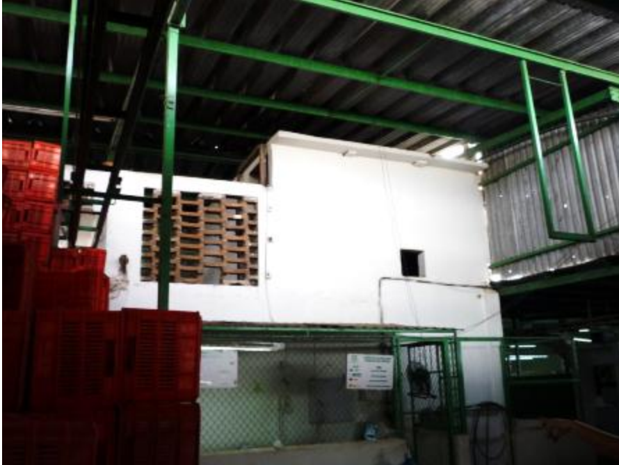
Figure 6-1 Old EDB fumigation chamber (currently used as a general shed) in a mango packinghouse in Escuinapa, Sinaloa, Mexico (Photo by author)
