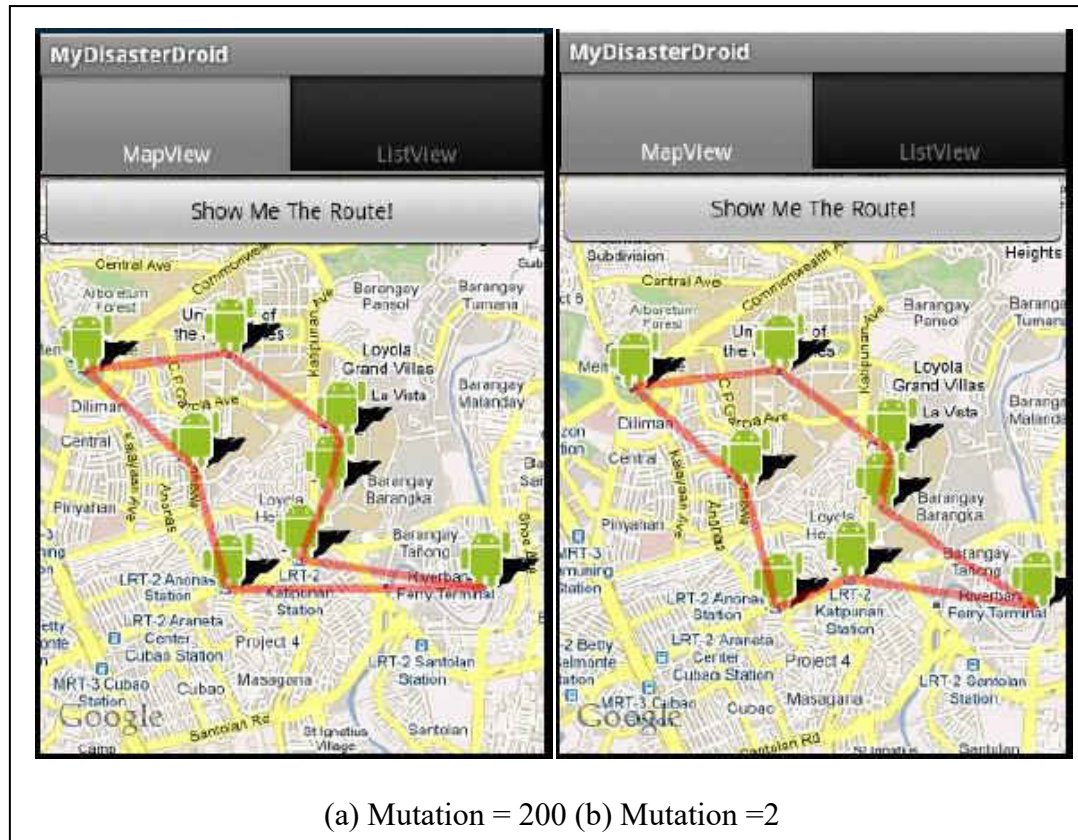
Figure 4-17 Path Calculation of MyDisasterDroid Project by GA Algorithm Source: Mobile Android based System. Http:// www.wseas.us/e-library/transactions/communications/2010/89-544.pdf
