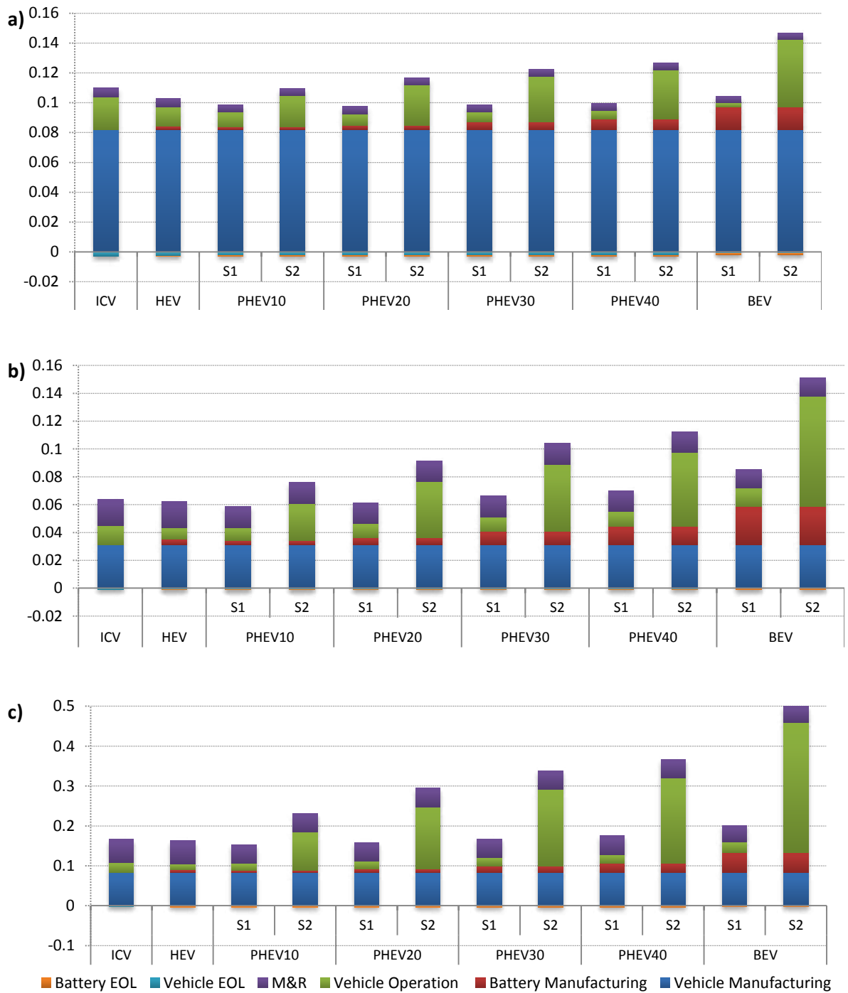
Figure 2 Economic impacts of alternative vehicle technologies: a) Foreign Purchase ($ per mile), b) Business Profit ($ per mile), c) GDP ($ per mile)
