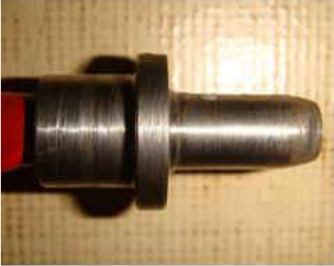
Figure 3.3: Corer-tipped bolt used for biopsy sampling of South African delphinids.
