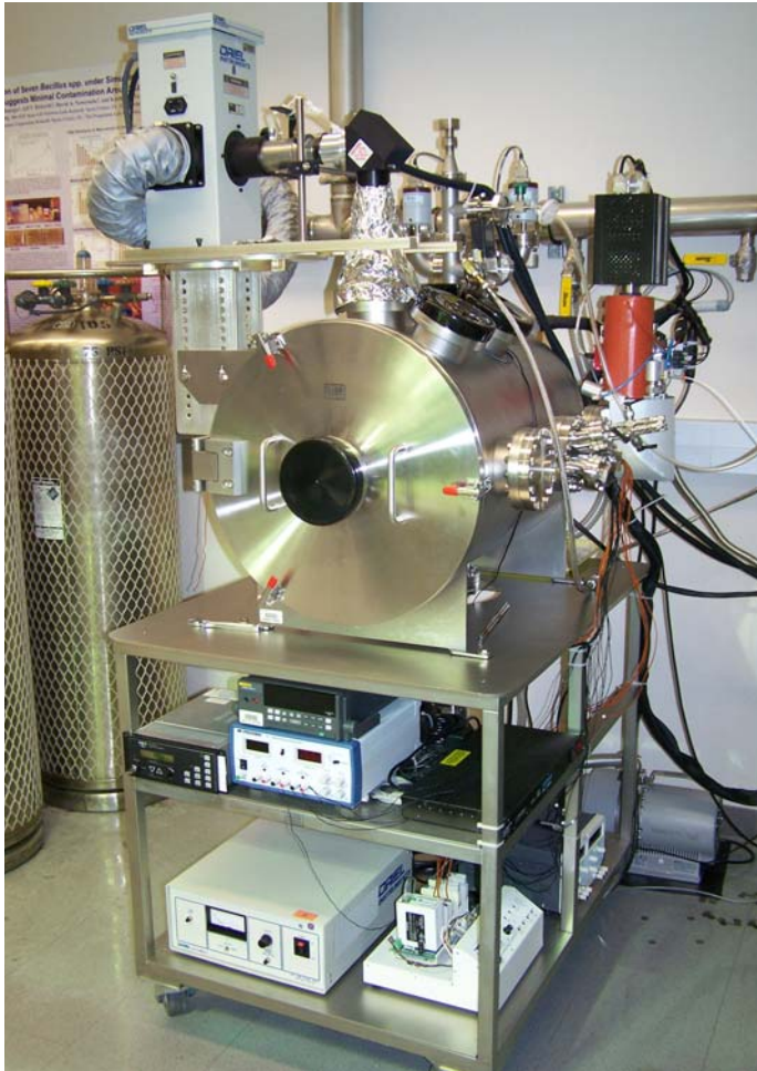
Figure 4. Mars Simulation Chamber. The MSC system can accurately simulate five key components of the surface environment of Mars including: (a) pressures down to 0.1 mb, (b) UV irradiation, (c) dust loading in the atmosphere, (d) temperature, and (e) a Mars atmosphere composed of CO 2 (95.3 %), N 2 (2.7 %), Ar (1.6 %), O 2 (0.13 %) and H 2 O (0.03 %).
