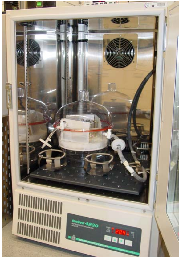
Figure 3. Low-pressure polycarbonate desiccator system used to reduce total atmospheric pressure down to 25 mb. Sterile in-line filters (0.2 \mu\text{m} pore-size) were added to the vacuum (right side) and venting (left side) lines. Four AnaeroPack pouches were placed within the desiccator to help scrub \text{O}_2 from the system.
