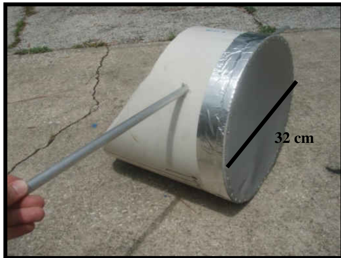
Figure 13: PVC plow 32 cm in diameter. Device used to make experimental propeller scars the same width, depth, and scar slope angle.
