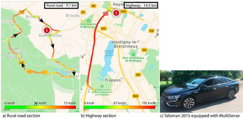
Figure 2. (a) rural road section (9.1 km), (b) highway section (14.5 km), (c) 2015 Renault Talisman equipped with Multi-Sense used in the experiment. The start/end is visualised with an S-sign, and the driven direction for the rural road is indicated with an arrow.
