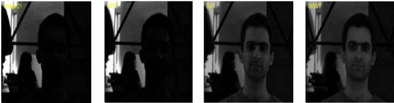
Figure 3.27: Left to right: Original image (person B11, image 21, completely shadowed), low-rank approximation using APG, SVT, and WSVT. WSVT removes the shadows and specularities uniformly from the face image especially from the eyes, chin, and nasal region.
