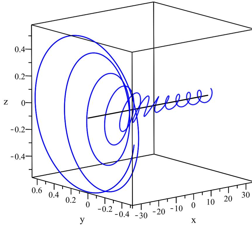
Figure 6.7: Plot of the deformed planar filament described by (6.58) when the temperature of the superfluid is  $T=1.5\text{K}$  ( $\alpha = 0.073$ ,  $\alpha' = 0.018$ ) and  $V = -1$ . The filament is given by numerically solving (6.59)-(6.60) subject to  $\phi(0) = 0.1$ ,  $\psi(0) = 0$ ,  $\phi'(0) = 0$ ,  $\psi'(0) = 0$ .
