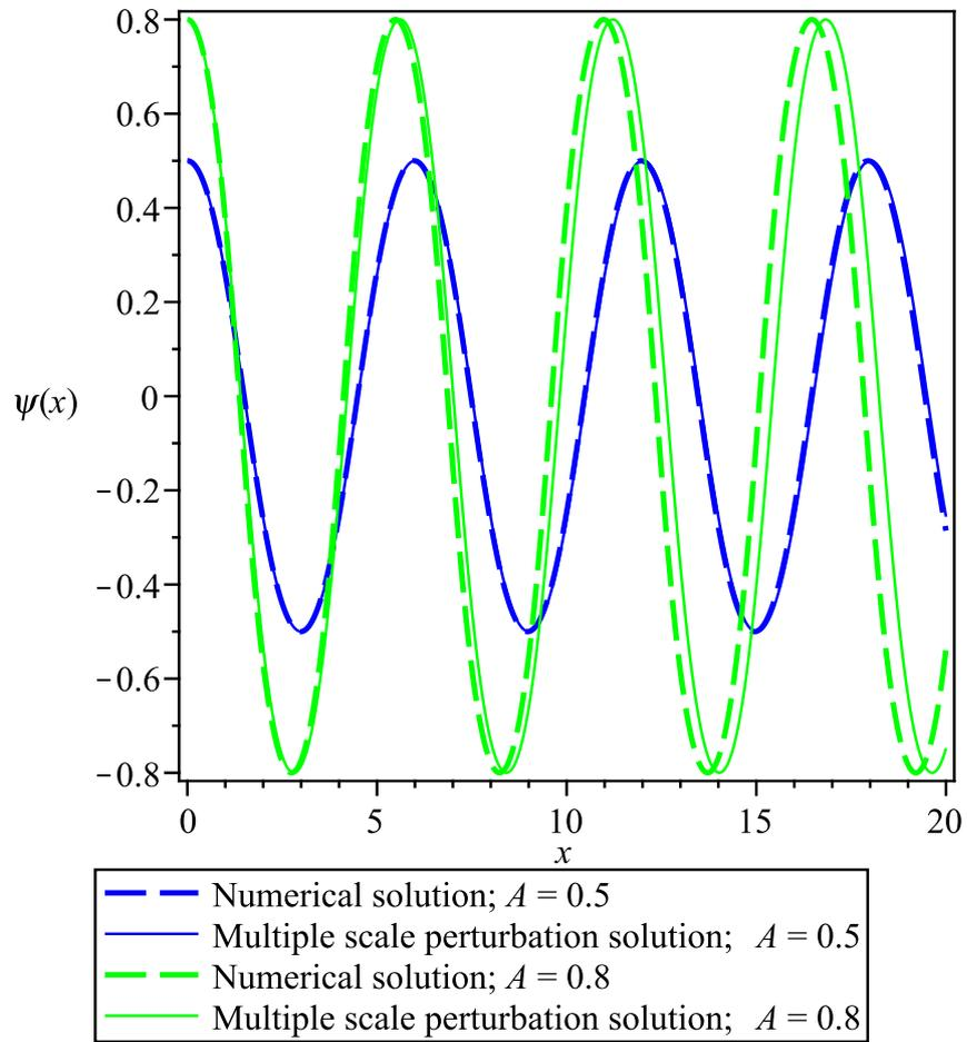
Figure 4.2: Plot of the perturbation solutions (4.20) for  $\psi(x)$  obtained through the method of multiple scales against numerical solutions obtained via the Runge-Kutta-Fehlberg method (RKF45) [29]. The valid region for the approximation (4.14) is  $A < 1/\sqrt{3} \approx 0.577$ , and in this region the results agree nicely. For larger  $A$ , the agreement breaks down, as the solutions fall out of resonance with the true solutions.
