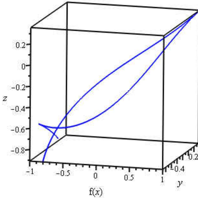
Figure 4.8: Plot of the numerical solution for a double loop vortex filament described by  $\phi(x)$  when  $\phi(x)$  satisfies (4.39),  $\phi(0.1) = 0.5$ ,  $\phi'(0.1) = -0.095$ . The  $x$  scaling is  $f(x) = \cos(x)$ . The space coordinate is parametrized by  $x \in [-4.0, 2.5]$ .
