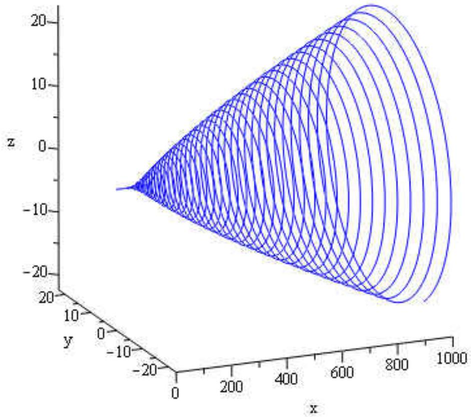
Figure 5.3: Vortex filament at temperature  $T = 1.5\text{K}$  we have  $\alpha = 0.073$  and  $\alpha' = 0.018$ .
