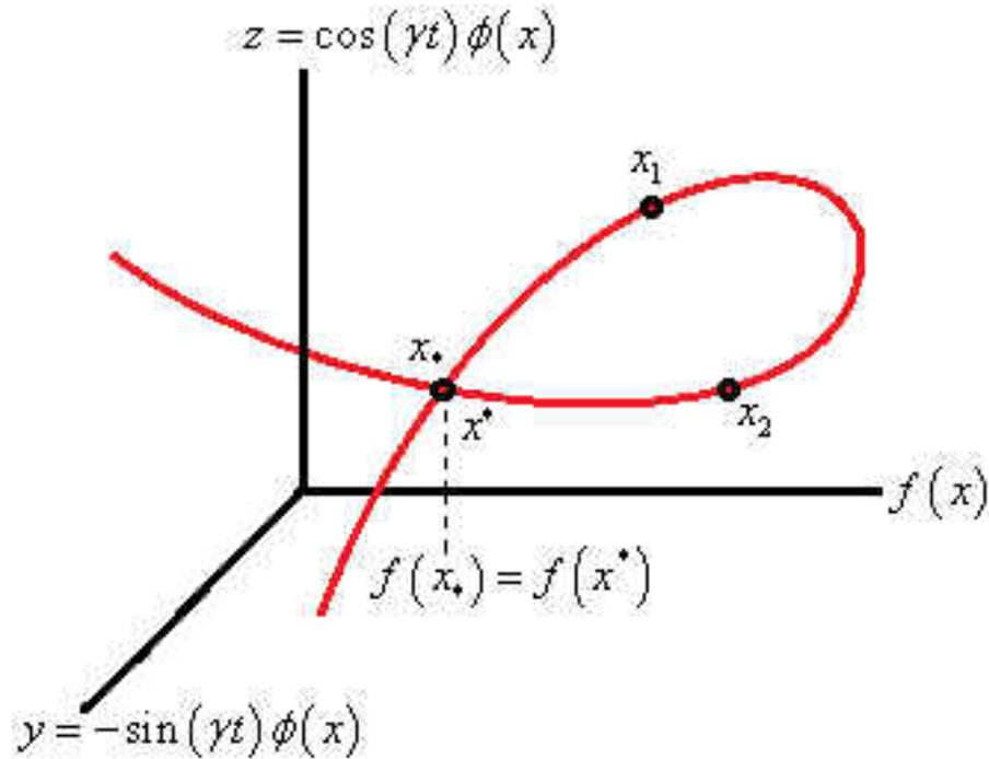
Figure 4.6: Schematic of a self-intersection for the planar vortex filament governed by a solution  $\phi(x)$  to equation (4.36). Self-intersection occurs at spatial coordinate  $f(x_*)$  where the parametrization  $x$  attains the value  $x^*$  such that  $f(x_*) = f(x^*)$  and  $\phi(x_*) = \phi(x^*)$ . It is necessary for  $\phi(x_1) \neq \phi(x_2)$  for all  $x_* < x_1 < x_2 < x^*$  in order to have a single loop. For multiple loops, similar yet more complicated conditions must hold.
