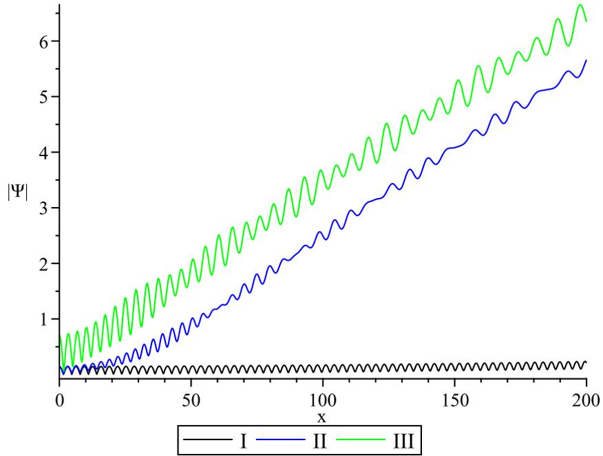
Figure 5.5: Plot of the modulus  $|\Phi| = \sqrt{\rho^2 + \sigma^2}$  given I:  $T = 1K$ ,  $\alpha = 0.005$ ,  $\alpha' = 0.003$ ,  $\rho(0) = \sigma(0) = 0.1$ ; II:  $T = 1.5K$ ,  $\alpha = 0.073$ ,  $\alpha' = 0.018$ ,  $\rho(0) = \sigma(0) = 0.1$ ; III:  $T = 1.5K$ ,  $\alpha = 0.073$ ,  $\alpha' = 0.018$ ,  $\rho(0) = \sigma(0) = 0.5$ . We set  $U_1 = \gamma = t = 1$ ,  $\rho'(0) = \sigma'(0) = 0$  in all plots. Note the intermittent behavior apparent in II and III.
