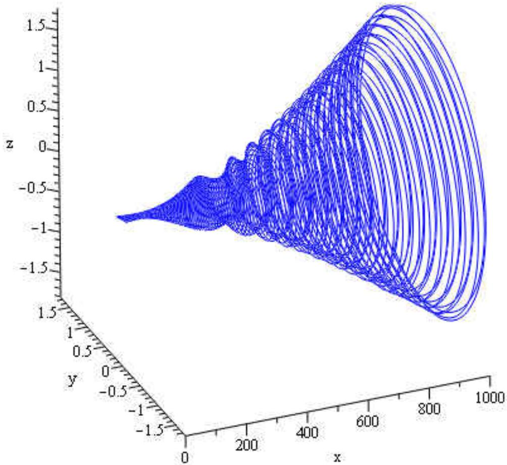
Figure 5.2: Vortex filament at temperature  $T = 1\text{K}$  where we have  $\alpha = 0.005$  and  $\alpha' = 0.003$ . We set  $U_1 = \gamma = t = 1$  and  $\rho(0) = \sigma(0) = 0.1$ ,  $\rho'(0) = \sigma'(0) = 0$ . Note the influence of the initial condition (compared with Fig. 5.1).
