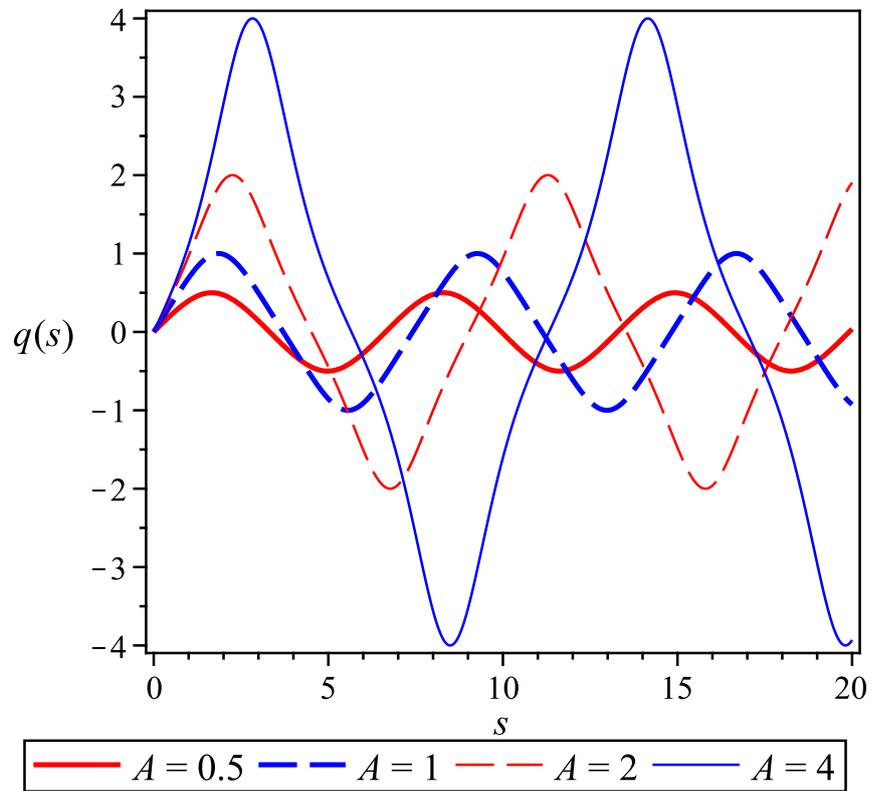
Figure 2.7: Plots of the solution  $q(s)$  given in (2.71) for various values of the amplitude  $A$ . Note that the period of the solutions is strongly influenced by the amplitude. The nonlinear dependence of the period  $T$  with the amplitude  $A$  is shown graphically in Fig. 2.8.
