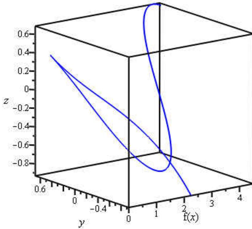
Figure 4.7: Plot of the numerical solution for a single loop vortex filament described by  $\phi(x)$  when  $\phi(x)$  satisfies (4.38),  $\phi(0.1) = 0.6$ ,  $\phi'(0.1) = -0.1$ . The  $x$  scaling is  $f(x) = x^2/2$ . The space coordinate is parametrized by  $x \in [-2.12, 3.00]$ .
