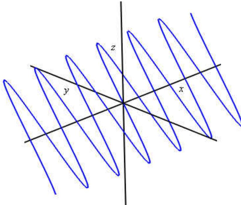
Figure 5.11: Schematic of the problem geometry for a planar vortex filament. The planar vortex filament is oriented along the  $x$ -axis, with radius  $A$  and  $x$ -period  $T(A)$ . The angular frequency,  $\omega = \gamma$  (by assumption (5.42)) determined the motion of the vortex filament with time. The temporal period is then  $2\pi/\gamma$ .
