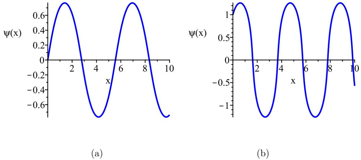
Figure 2.2: Plots of  $\psi(x)$  when  $\psi(0) = 0$  (a),  $1$  (b), while  $\psi'(0) = 1$ .
