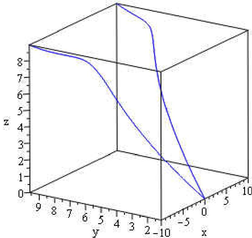
Figure 4.14: Time evolution of a vortex filament kink solution of the type described by (4.69). We set  $t = 10$ , and we have taken  $C = 1 + i$ ,  $\gamma = 1$ ,  $\epsilon = 0.25$ . While oscillations initially appear along the filament, these die off as time becomes large, and therefore the filament tends to the limit (4.72) as time grows.
