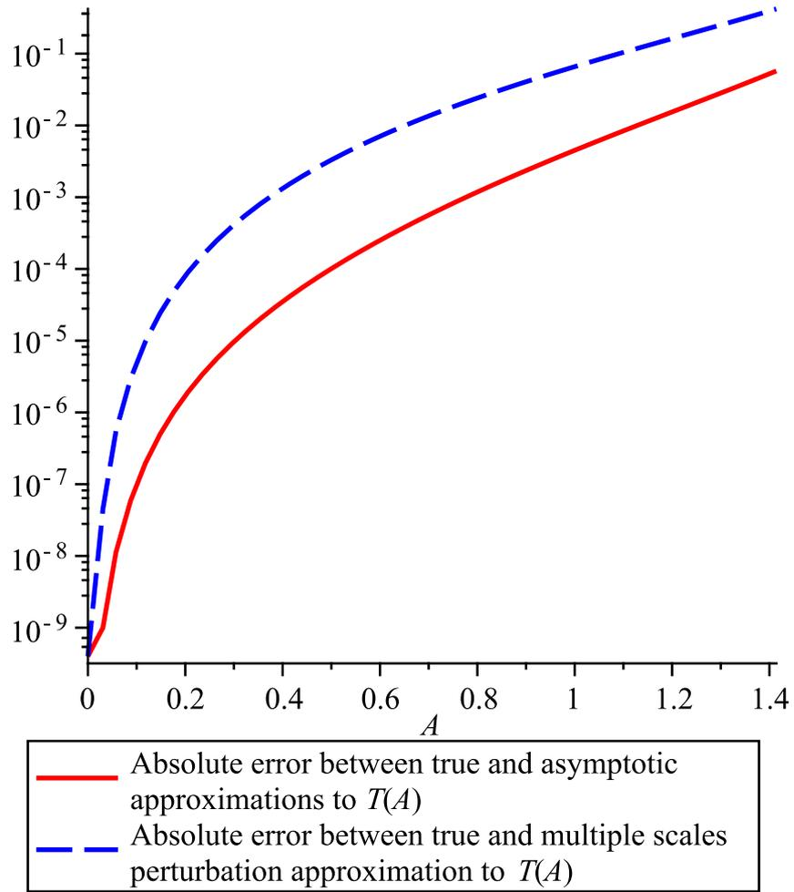
Figure 4.5: We demonstrate the relative error between the approximations to the period  $T(A)$  and the true solution (4.29). Both are extremely accurate for small  $A$ , and gradually lose accuracy for larger  $A$ , though the asymptotic approximation (4.32) outperforms the multiple scale approximation (4.21) nicely. That said, in its region of validity ( $A < 1/\sqrt{3}$ ), the multiple scale approximation (4.21) is rather accurate for only a first order perturbation result.
