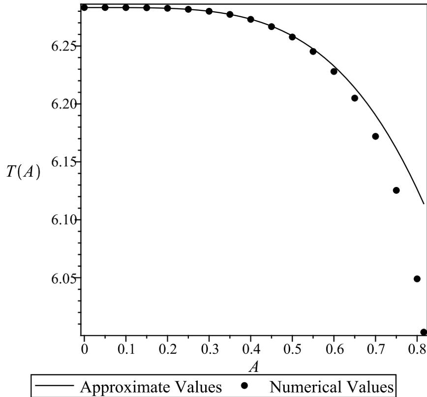
Figure 5.12: Plot of the approximation (5.54) to the space period  $T(A)$  of the planar vortex filament given by the method of multiple scales. Also plotted are the exact numerical values for  $T(A)$  that may be found by numerically integrating (5.44) in order to construct a solution. Clearly, the multiple scales approximation is a very good fit for small-amplitude solutions. Periodic solutions exist for  $A < \sqrt{2/3} \approx 0.81649$ .
