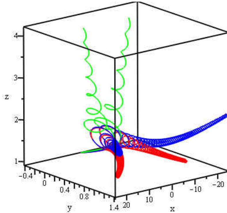
Figure 5.15: Plot of singular self-similar solutions  $\hat{\mathbf{r}}$  for (5.63)-(5.64). The red (lower) solution denotes  $(\alpha, \alpha') = (0, 0)$ , the blue (middle) solution denotes  $(\alpha, \alpha') = (0.005, 0.003)$ , and the green (upper) solution denotes  $(\alpha, \alpha') = (0.073, 0.018)$ . Here  $R(0) = 1$ ,  $R'(0) = \Theta'(0) = 0$ ,  $\Theta(0) = 2$ .
