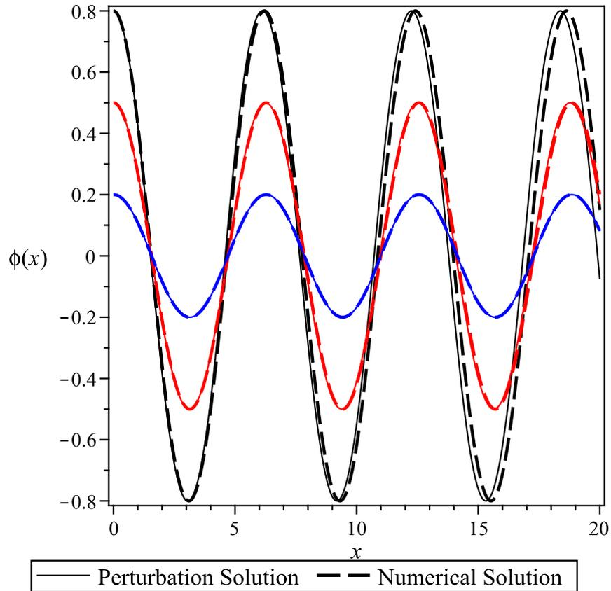
Figure 5.13: Plot of the space periodic part of the planar vortex filament, for various values of  $A$ . Solid lines denote the perturbation approximation (5.53) while the dashed lines denote numerical simulations via RKF45 method of numerical integration. We see remarkable agreement for small amplitude solutions. For the large amplitude solutions, the numerics and analytics begin to go out of phase for large  $x$ , due to the small error in the approximate period (5.54) and the true period.
