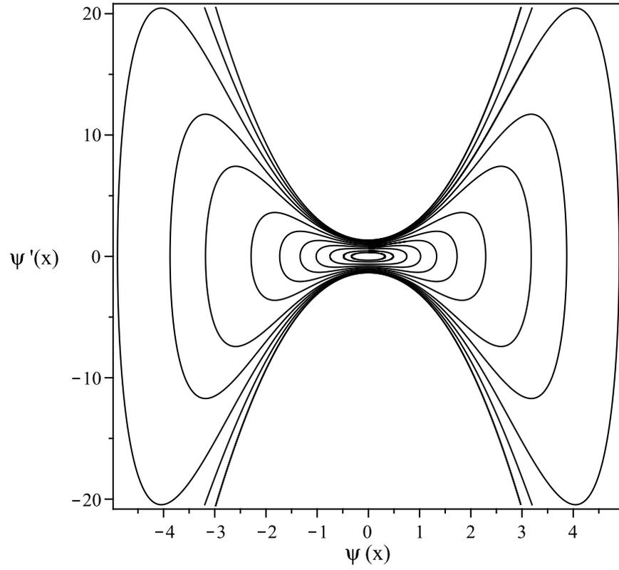
Figure 2.10: Phase portraits for the space-periodic solutions  $\psi(x)$  to the WKIS equations, which exist for  $-1 < I < 0$ . We fix  $k = 1$ .
