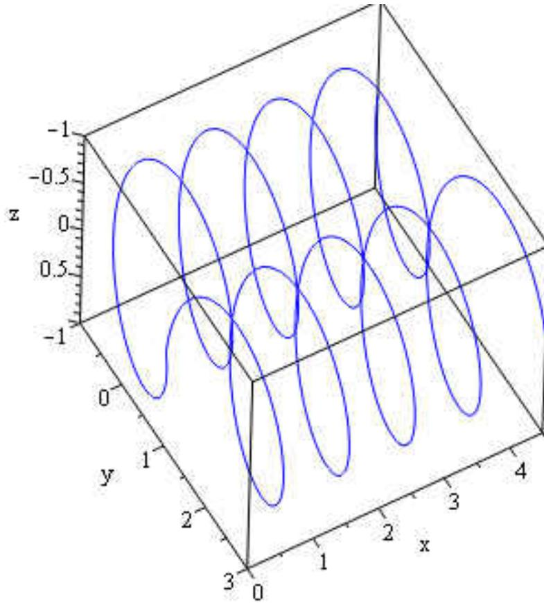
Figure 4.12: A vortex filament loop formed at  $t = 0$  by two scaled helical vortex filament segments as defined in (4.65). Before  $t = 0$ , the two filament sections do not form a closed loop, and for  $t > 0$  the filaments separate and the loop is broken. Therefore, the loop is a highly localized temporal event. The loop can redevelop at a later time. Here the scaling is  $\mu(x) = \cos(x)$ , and to illustrate the results graphically we take  $k = 2\pi$ ,  $A = 1$ ,  $\gamma = 1$ .
