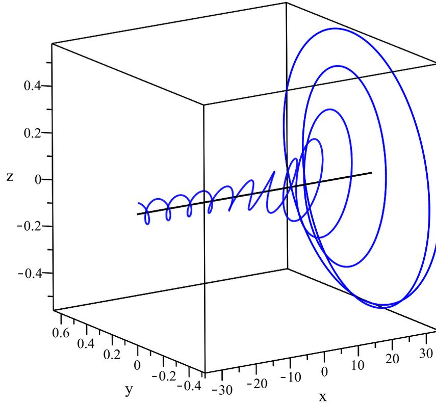
Figure 6.6: Plot of the deformed planar filament described by (6.58) when the temperature of the superfluid is  $T=1.5\text{K}$  ( $\alpha = 0.073$ ,  $\alpha' = 0.018$ ) and  $V = 1$ . The filament is given by numerically solving (6.59)-(6.60) subject to  $\phi(0) = 0.1$ ,  $\psi(0) = 0$ ,  $\phi'(0) = 0$ ,  $\psi'(0) = 0$ .
