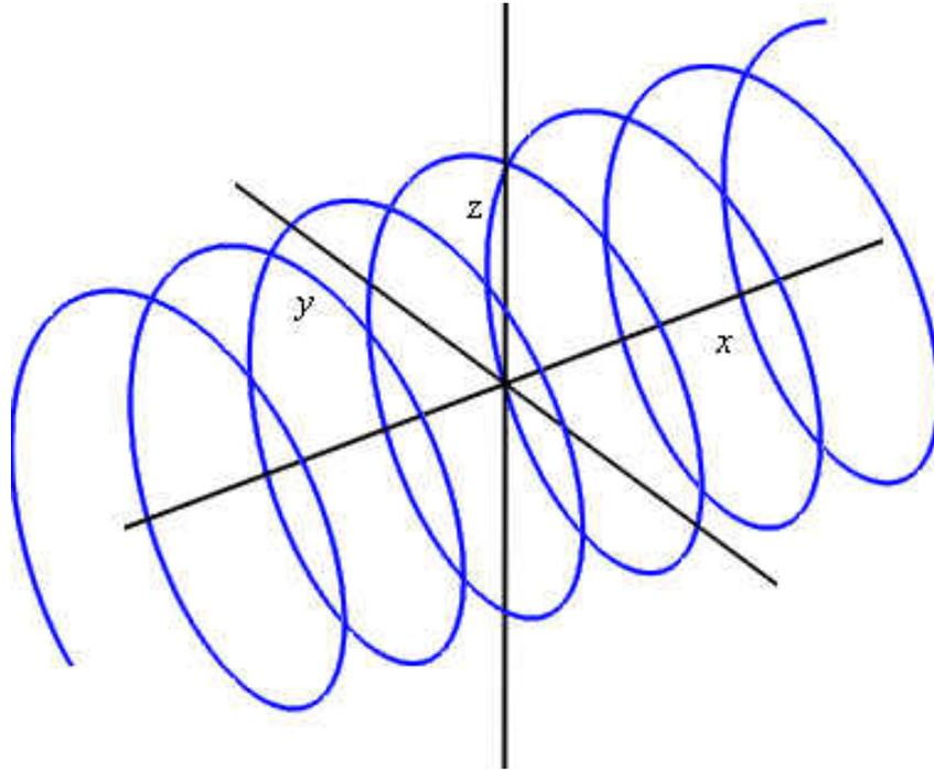
Figure 5.8: Schematic of the problem geometry for a prototypical helical vortex filament. The helical vortex filament is oriented along the  $x$ -axis, with amplitude  $A$  and wave-number  $k$ . The angular frequency,  $\omega$ , will dictate the motion of this helical vortex filament.
