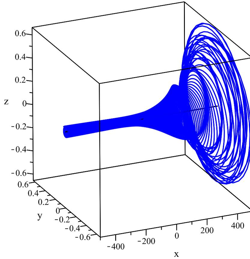
Figure 6.5: Plot of the deformed planar filament described by (6.58) when the temperature of the superfluid is  $T=1\text{K}$  ( $\alpha = 0.005$ ,  $\alpha' = 0.003$ ) and  $V = 1$ . The filament is given by numerically solving (6.59)-(6.60) subject to  $\phi(0) = 0.1$ ,  $\psi(0) = 0$ ,  $\phi'(0) = 0$ ,  $\psi'(0) = 0$ .
