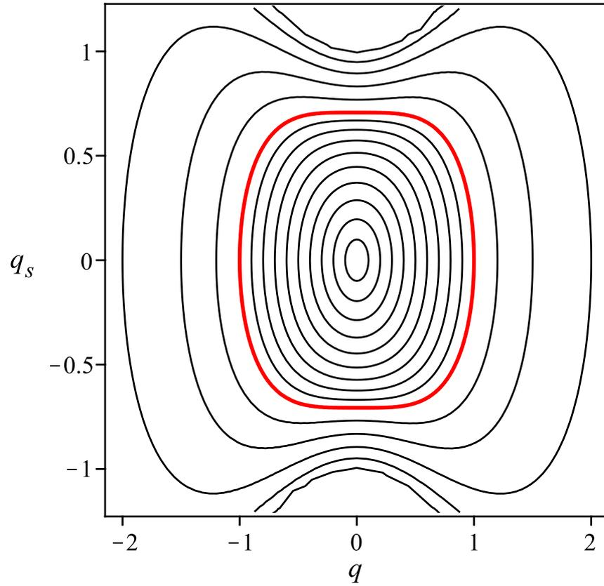
Figure 2.6: Phase portrait in  $(q, q_s)$  for the solution to the fully nonlinear oscillator equation modelling the local induction equation under the arclength representation.
