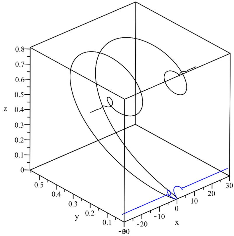
Figure 5.21: Soliton solutions (5.134) are given in (d), for  $\alpha = 0.005$  (black line) and  $\alpha = 0.073$  (blue line) in the presence of a normal fluid ( $U = 1$ ). The perturbation size of these soliton excitations of the tangent filament is  $\epsilon = 0.01$  (though the corresponding value of the perturbation is much larger in the Cartesian frame).
