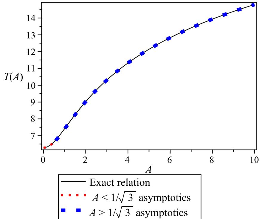
Figure 2.8: Plot of the period  $T(A)$  of the solution (2.71) versus the amplitude  $A$ . The exact relation is found by numerically plotting (2.72). Note that both the  $A < 1/\sqrt{3}$  and  $A > 1/\sqrt{3}$  asymptotic expansions are excellent fits to the exact relation.
