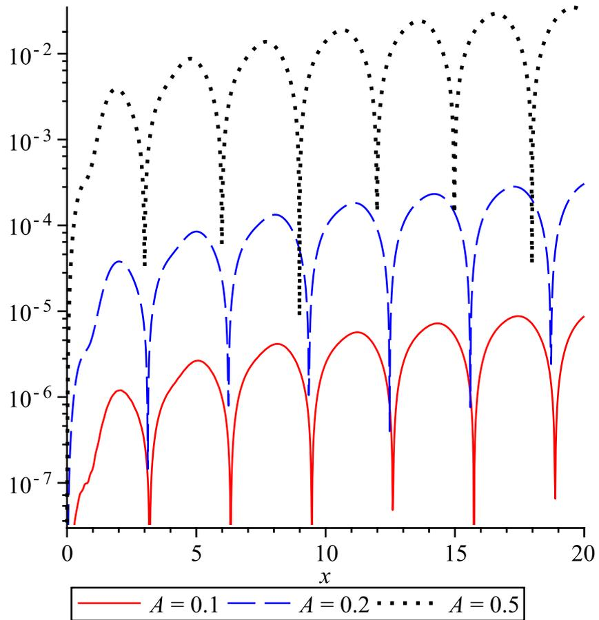
Figure 4.3: Plot of the absolute error between the perturbation solutions (4.20) for  $\psi(x)$  obtained through the method of multiple scales and the numerical solutions obtained via the Runge-Kutta-Fehlberg method (RKF45) [29]. The agreement is strong for small amplitude solutions, while the agreement gradually breaks down for larger amplitudes.
