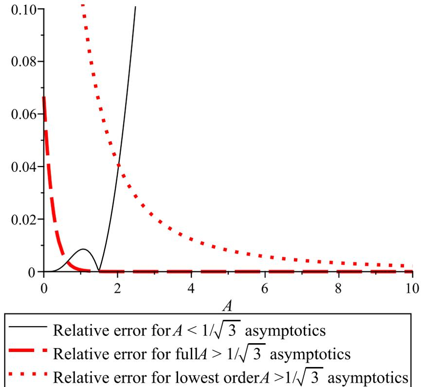
Figure 2.9: Relative error  $|T(A) - T_{\text{approx}}|/|T(A)|$  of the approximations to  $T(A)$ . We also include the lowest order approximation  $T(A) \approx 4 \ln(2\sqrt{2m})$  for the  $A > 1/\sqrt{3}$  case. We see the good agreement with the  $A < 1/\sqrt{3}$  asymptotics and  $A > 1/\sqrt{3}$  asymptotics where needed.
