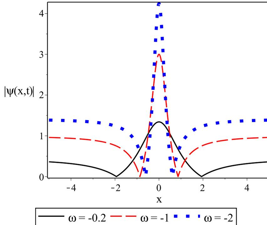
Figure 3.6: Influence of the spectral parameter,  $\omega < 0$ , on the wave envelopes. As  $|\omega|$  increases, the amplitude increases like  $3\sqrt{|\omega|}$  yet the mass of the wave remains fixed. Hence, a greater proportion of mass is allocated near the center of the wave, in the case of large amplitude solitons. Note that by amplitude, we refer to deviation of the mean wave-height (which is  $\sqrt{|\omega|}$ ) - the total height of the wave, in this model, is  $4\sqrt{|\omega|}$ .
