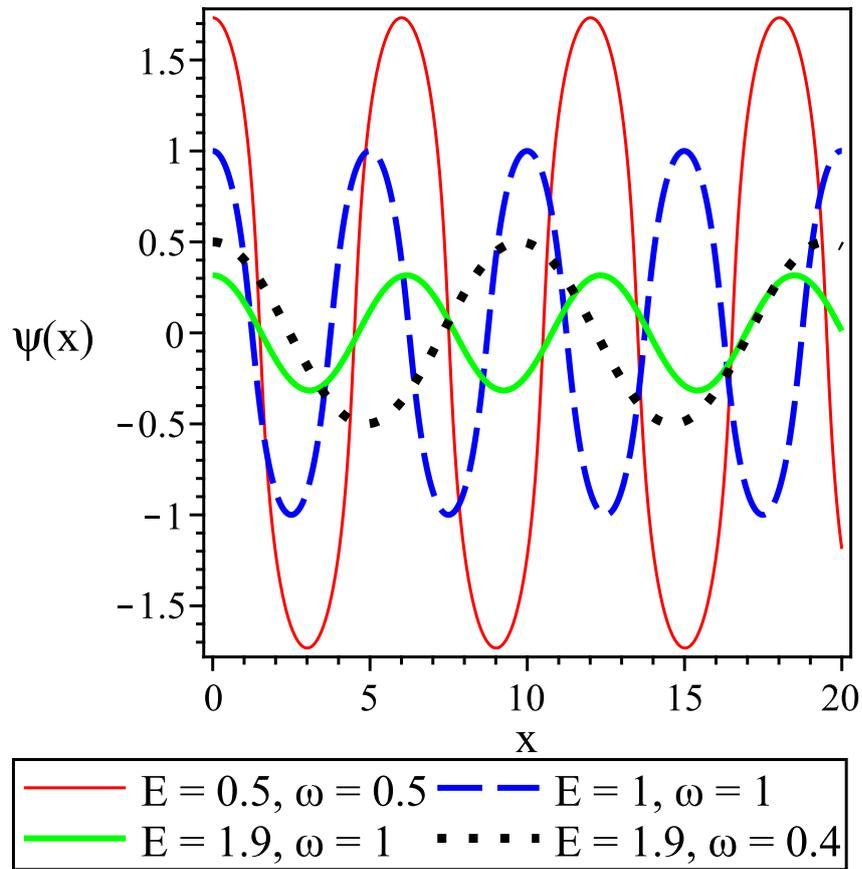
Figure 3.2: Plot of the solution profiles  $\psi(x)$  with spectral parameter  $\omega$  and constant of motion  $E$ . Clearly, both parameters strongly influence the amplitude and space-period of the stationary solutions. Each stationary solution  $\psi(x)$  corresponds to a planar vortex filament as shown in Fig. 3.1.
