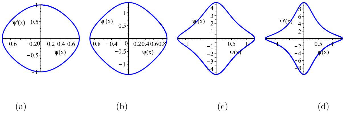
Figure 2.1: Phase portraits for  $\psi(x)$  when  $\psi(0) = 0$  (a),  $0.5$  (b),  $1$  (c),  $1.1$  (d) while  $\psi'(0) = 1$ .
