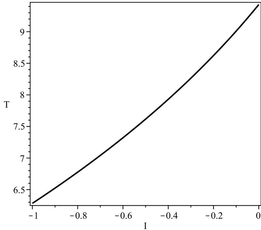
Figure 2.12: Plot of the period  $T$  of the space-periodic solutions  $\psi(x)$  to the WKIS equation for various values of the constant of motion  $I$ . Here,  $k = 1$ .
