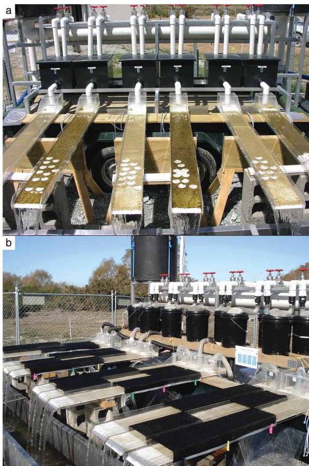
Fig. 4. The experimental flume apparatus used during the collaborative research project between EC and NIWA during 2008–2010 was located on the bank of the Waitaki River, South Island, New Zealand, adjacent to the confluence with the Otiake Spring Creek. (a) The initial design in 2008 had six flumes, all initially colonized with D. geminata using Waitaki River water. Subsequently, three of the flumes were shifted to Otiake Spring Creek water (treatment), while the other three remained as controls and continued to receive Waitaki River water (details in Bothwell & Kilroy 2011). (b) In 2009–2010, a total of 12 flumes were employed to test additions of P or N and light intensity using shading cloth (details in Bothwell & Kilroy 2011; Kilroy & Bothwell 2011a).
