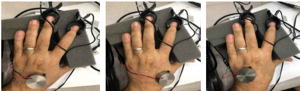
Figure 79: Experimental set up, sensors and exciter location for system miniaturization experiment. Case 1, 2, and 3 are shown from left to right in the Figure.
