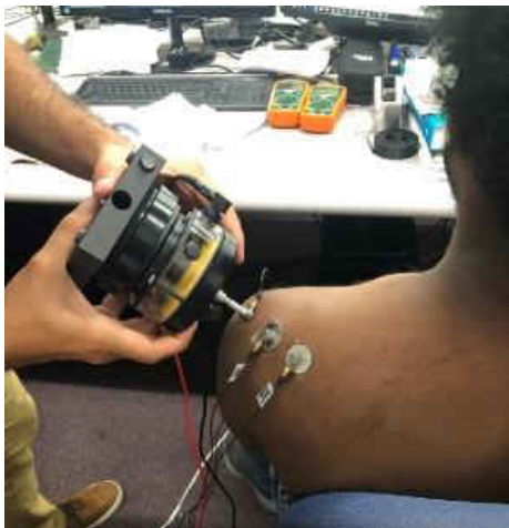
Figure 13: Experimental set up for testing the effect of static force loading in humans
