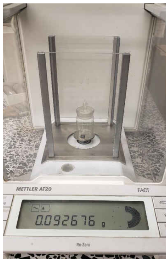
Figure 7. Mass determination of each o-ring based on ASTM procedure.
