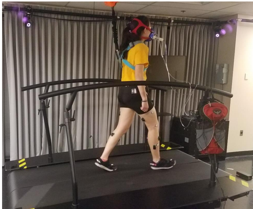
Figure 4: Experiment set up with subject walking on treadmill while metabolic and motion capture data is collected
