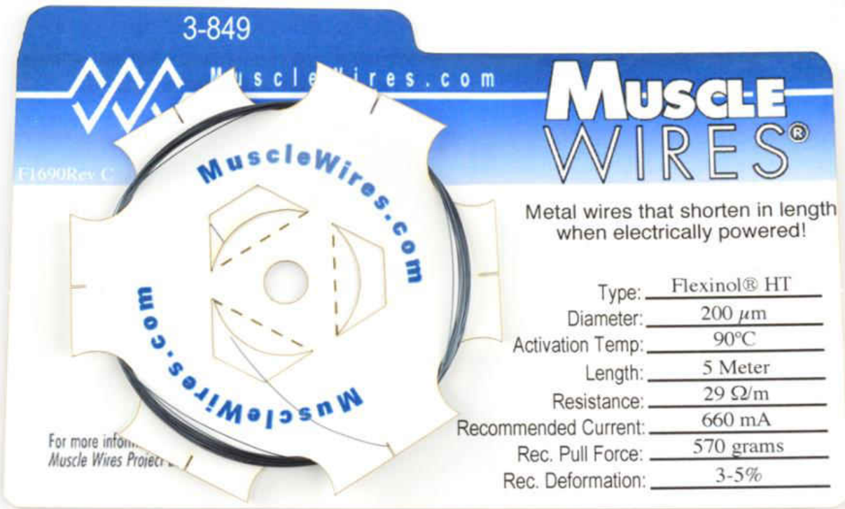
Figure 13 SMA wire sample by Flexinol with specifications listed on the packaging [15].
