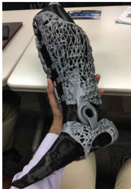
Figure 41. ML optimized cast provided by Stratasys
