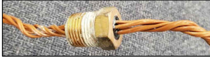
Figure 4-8 Thermocouple feedthrough used in evaporator/condenser chamber
