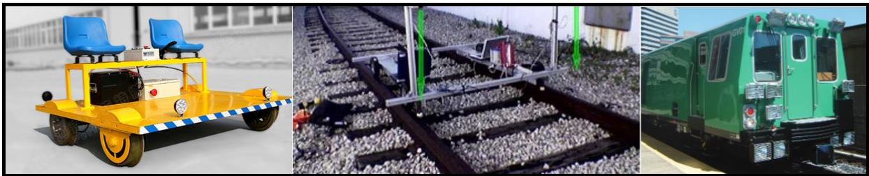
Figure 1 Various platforms for railroad inspection
