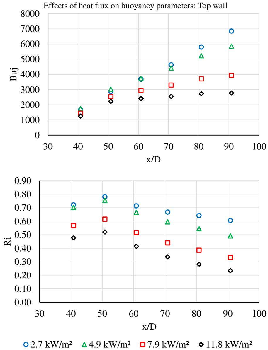
Figure 5.13: Variation in buoyancy parameters with heat flux at top wall
