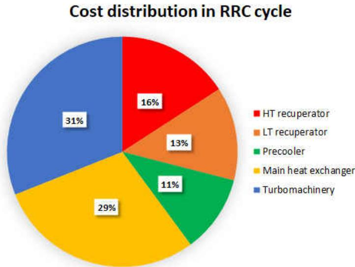
Figure 1.3: Cost distribution in RRC cycle plotted from cycle optimization study [1] showing cost of heat exchangers as majority
