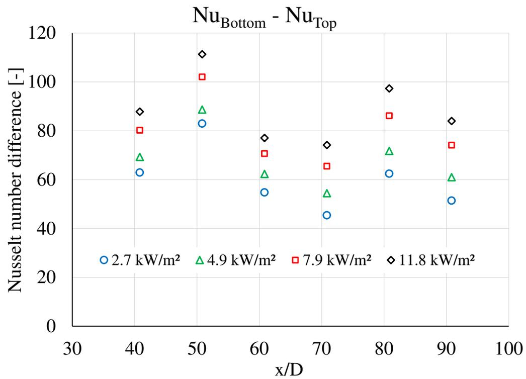
Figure 5.12: Difference in Nusselt number at bottom and at top wall location with heat fluxes
