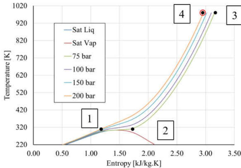
Figure 1.5: Temperature-Entropy diagram for CO<sub>2</sub> (1, 2, 3, 4 are four states, not necessarily corresponding to a thermodynamic cycle)
