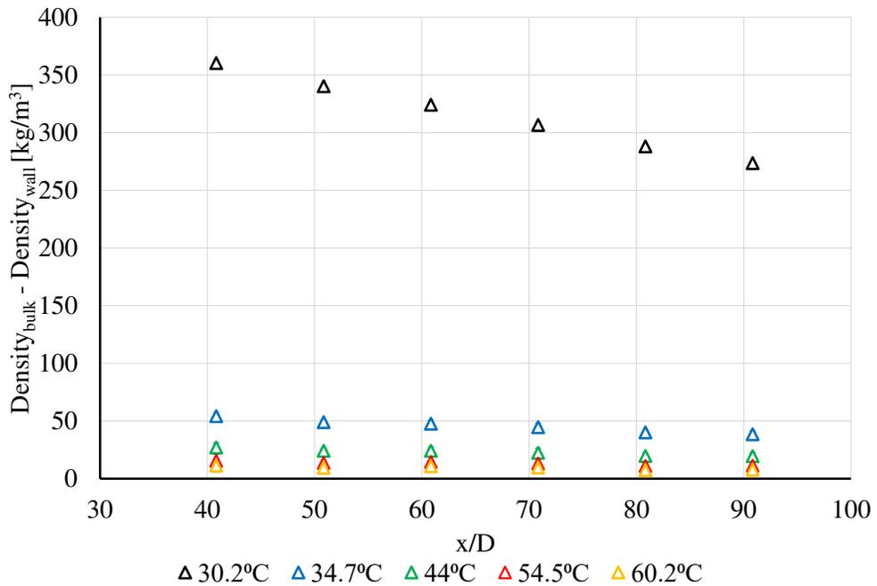
Figure 5.16: Difference between density at wall and bulk fluid density at different inlet temperature conditions
