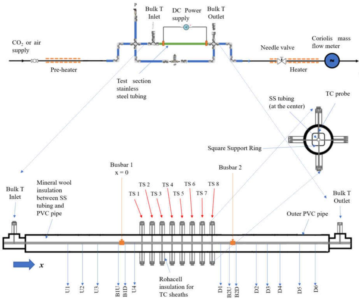
Figure 4.1: Schematic of experimental setup in open loop (top) and details of instrumented test section (bottom)
