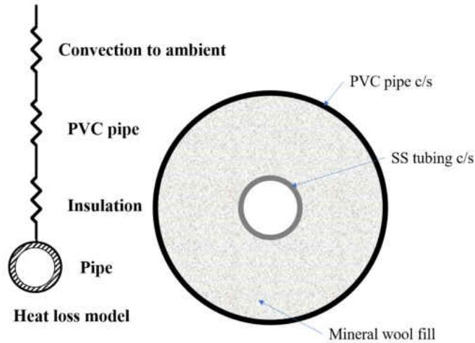
Figure 4.2: Pathway for radial heat loss to ambient
