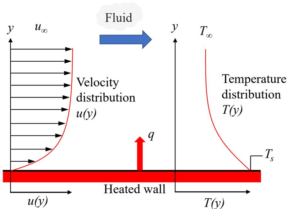
Figure 5.1: Boundary layer development on heated wall surface
