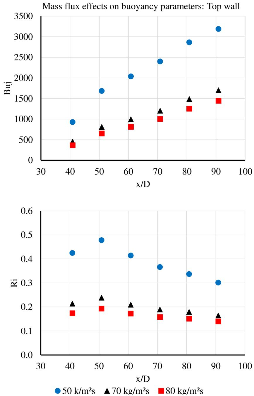
Figure 5.9: Variation in buoyancy parameters with mass flux at top wall
