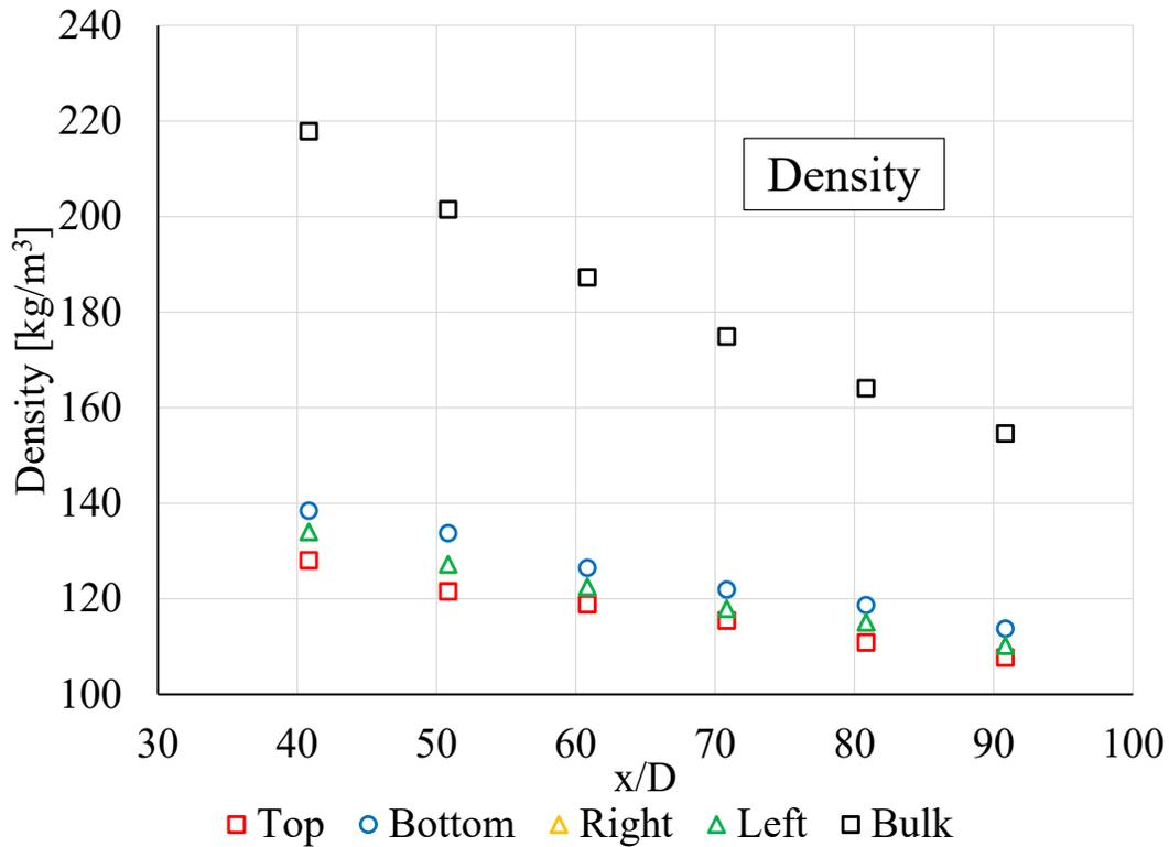
Figure 5.5: Circumferential variation in density plotted for case HF4 as listed in Table 5.3
