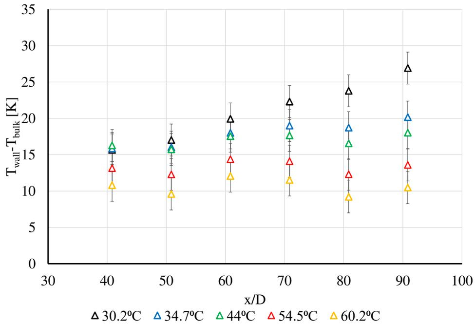
Figure 5.15: Difference between wall temperature and bulk temperature at different inlet temperature conditions
