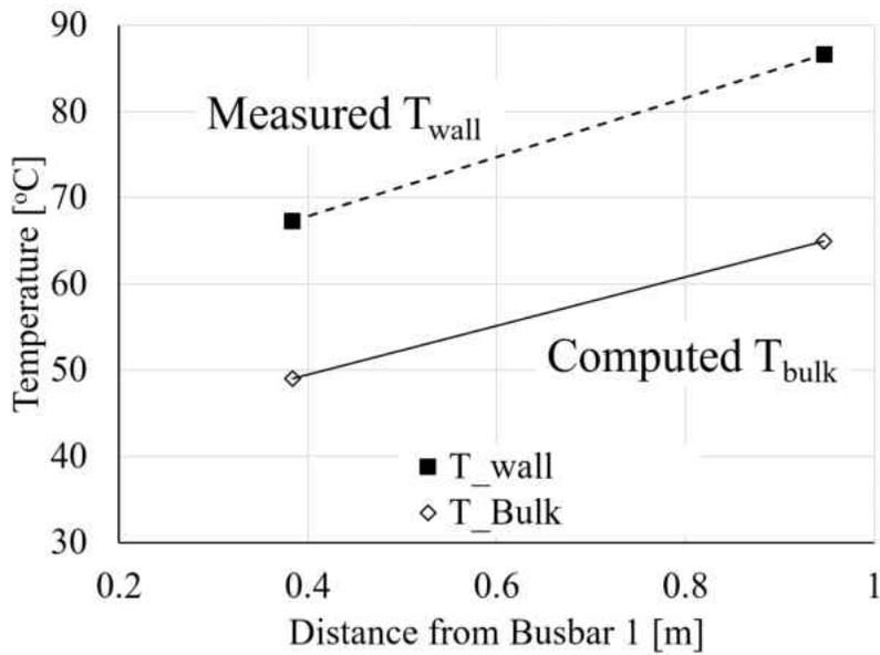
Figure 4.5: Wall temperature vs Bulk flow temperature comparison for air validation case 7 (as mentioned in Table 4.4)
