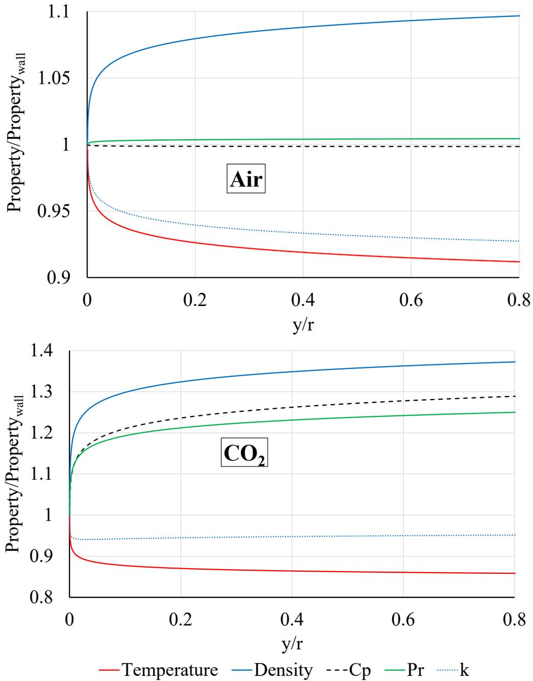
Figure 5.3: Profile of properties as ratio to properties at wall according to thermal law of the wall: Top- air validation case 7 as shown in Table 4.4, Bottom- case HF4 as shown in Table 5.3
