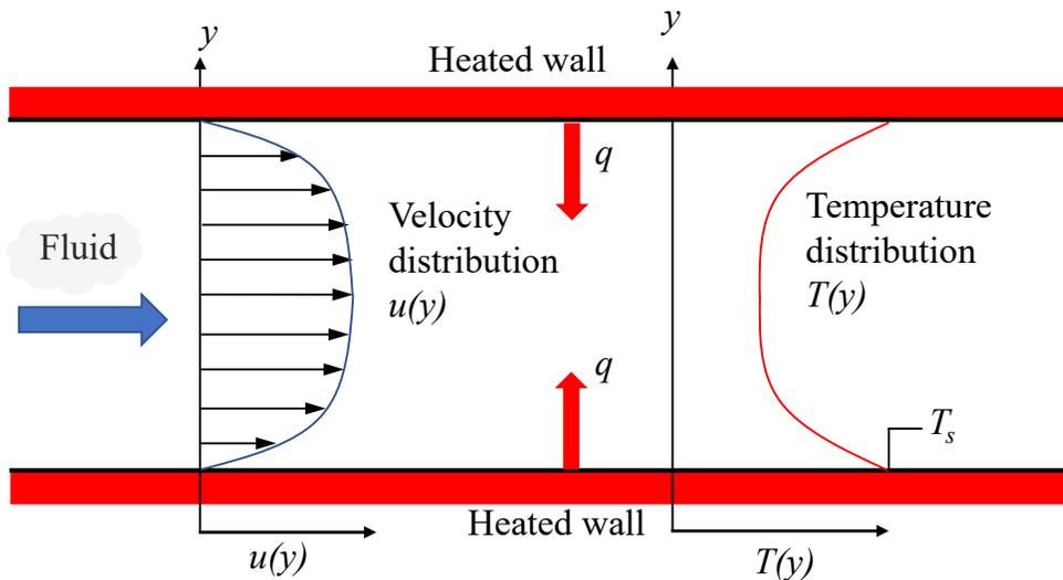
Figure 5.2: Boundary layer development on heated wall surface for internal flow
