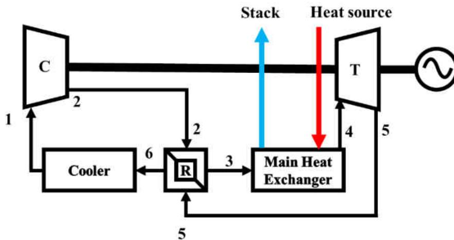
Figure 1.1: Recuperated configuration of Brayton cycle
