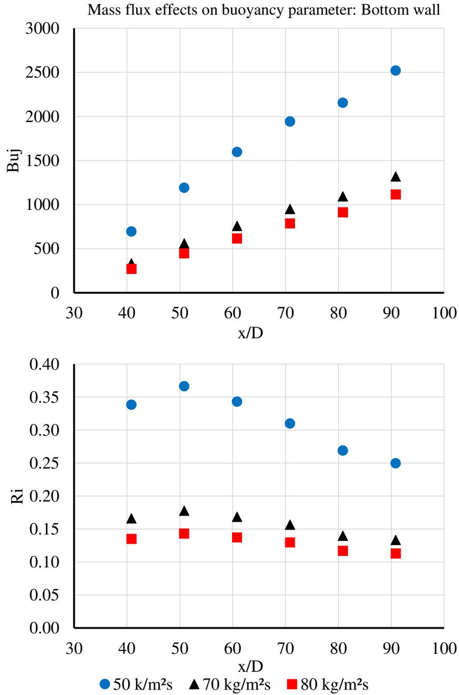
Figure 5.10: Variation in buoyancy parameters with mass flux at bottom wall
