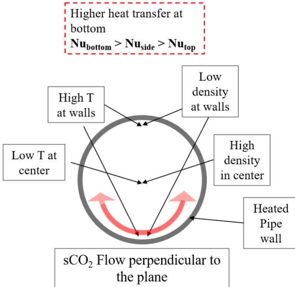
Figure 5.7: Schematic of cross section of tube showing natural convection current from bottom wall to top wall (CO<sub>2</sub> flow direction going into the page)
