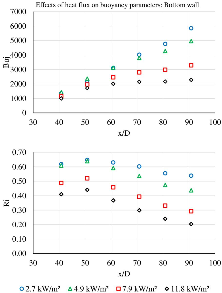
Figure 5.14: Variation in buoyancy parameters with heat flux at bottom wall
