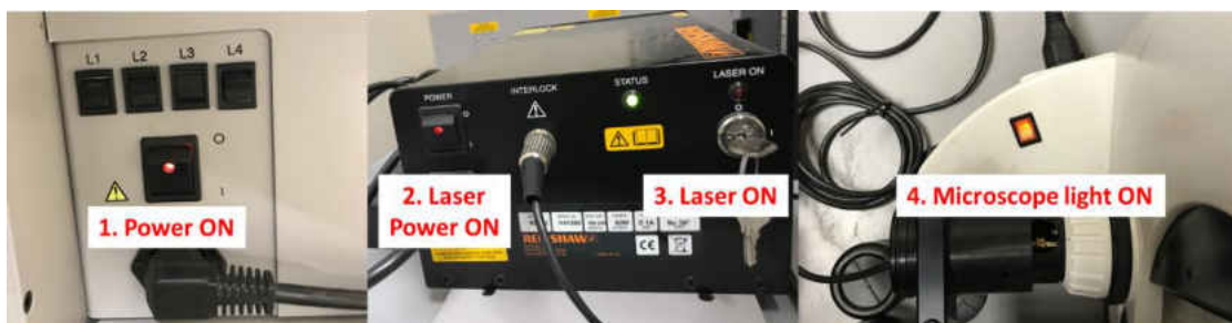
Figure 62: Raman spectrograph machine power on procedure.
