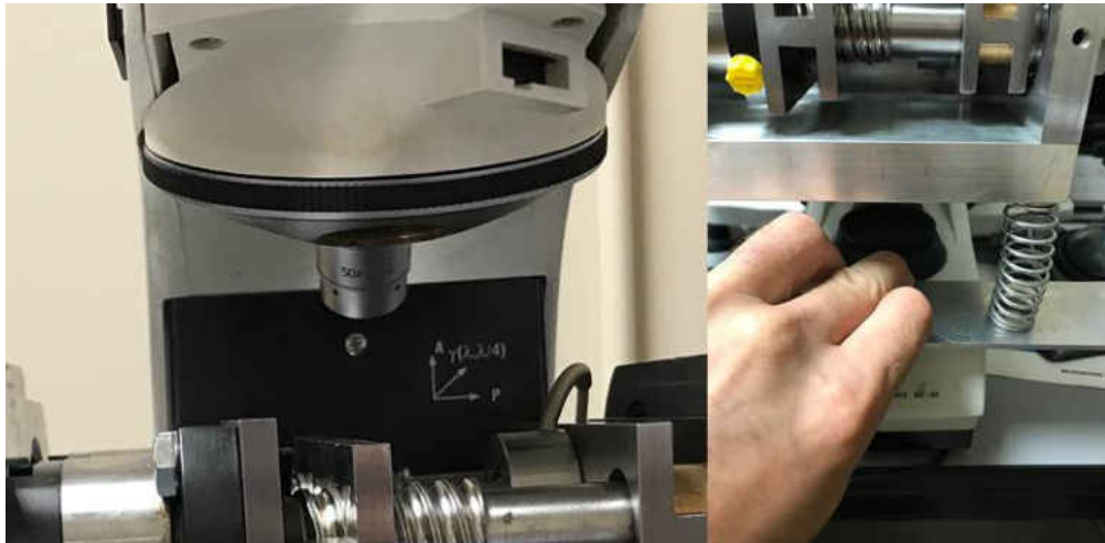
Figure 63: Microscope lens in rear position and removing stage support springs.
