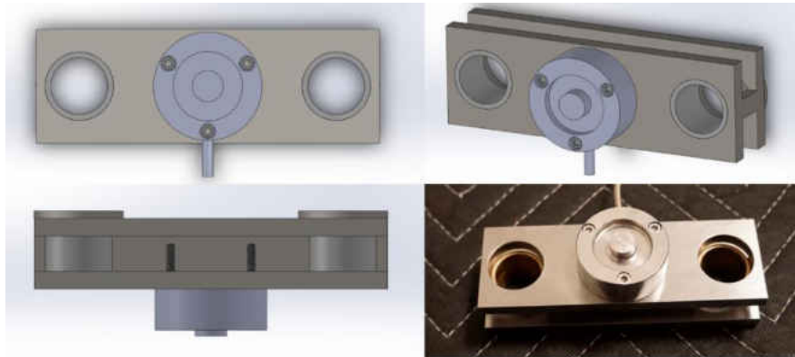
Figure 37: Support crosshead subassembly.
