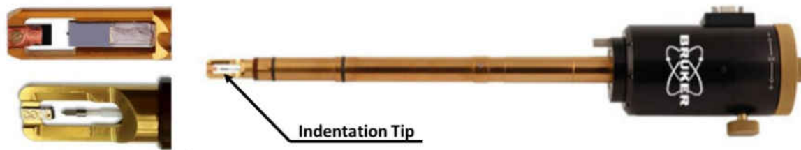
Figure 10: Hysteron PI 95 TEM Pico indenter with close of loading tip [22].
