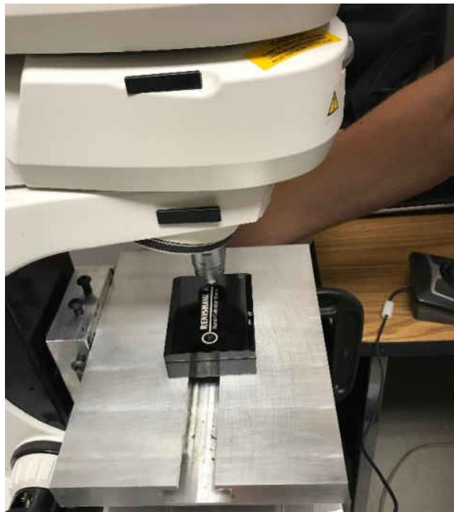
Figure 64: Calibration sample stage and calibration reference sample.
