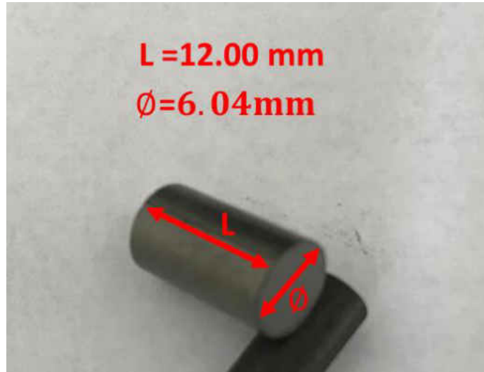
Figure 26: \text{LaCoO}_3 cylindrical ceramic sample used for testing with a diameter of 6.04mm.
