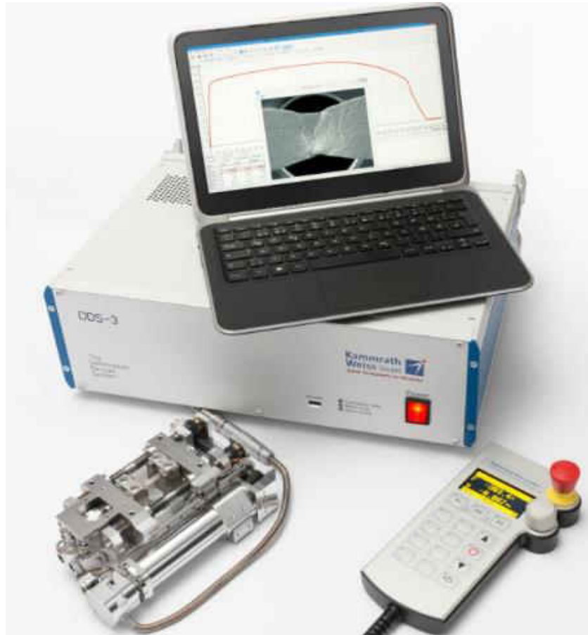
Figure 21: The Kammrath and weiss tensile and compression module [29].
