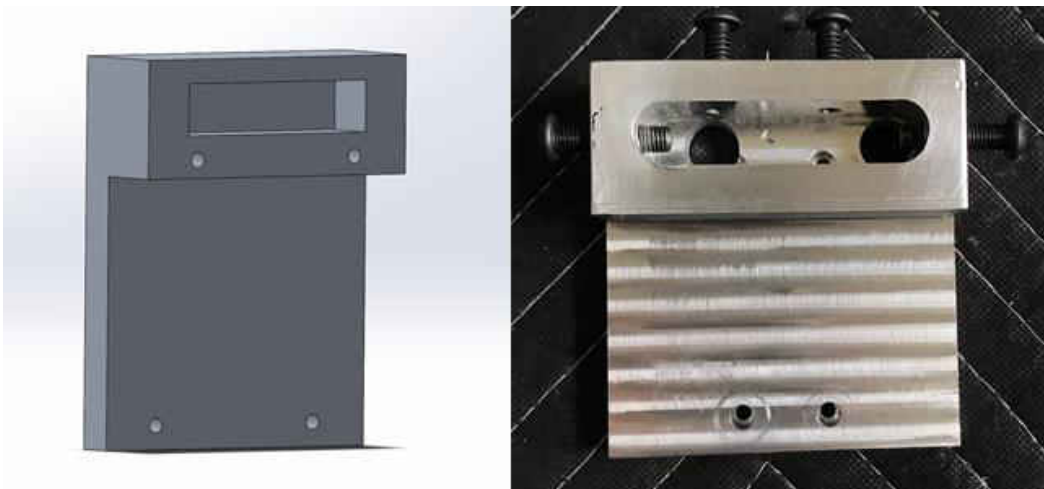
Figure 41: Compression stage mounting fixture.
