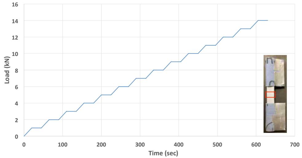
Figure 3.8: A load step plot showing when displacement holds were implemented to perform the PS map scans. Displacement holds were done at 1 kN load increments, and the samples were taken up to 14 kN.
