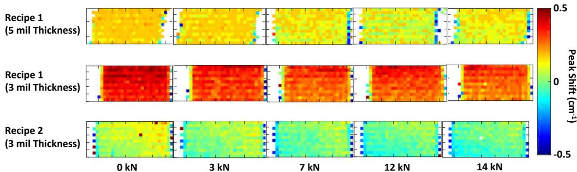
Figure 3.10: Comparisons of the stress states with increasing uniaxial tensile load of paint-based PS coatings with different thicknesses (5 mil and 3 mil) and different processing recipes (1 and 2) that qualitatively show leftward R1 peak shifts from the unloaded condition.
