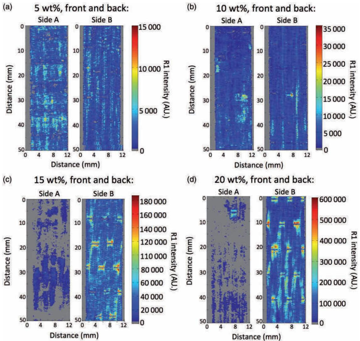
Figure 1.3: Intensity maps showing dispersion of alumina particles within HCFRPs of varying particle content [2].
