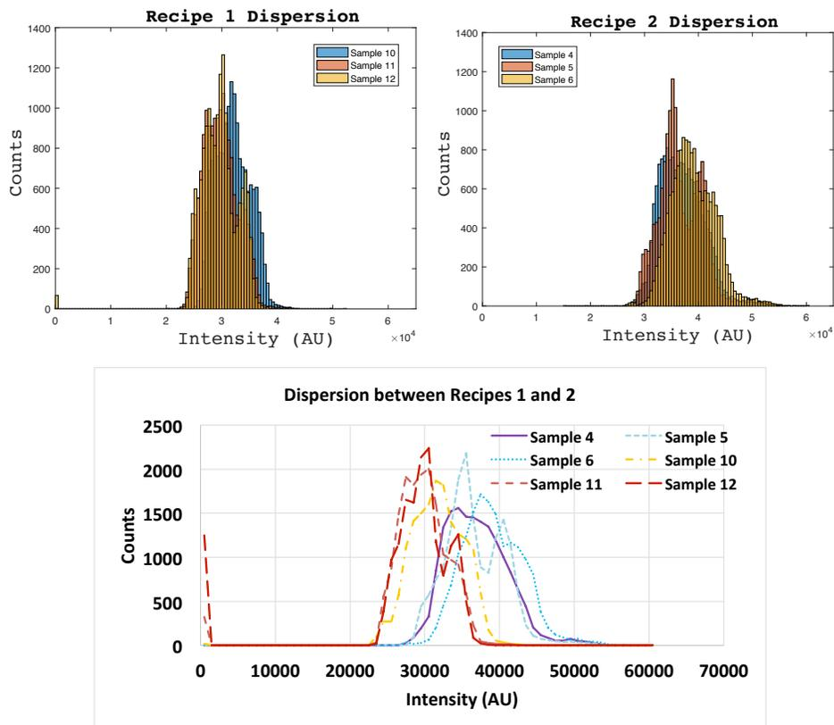
Figure 3.7: Histograms were plotted to show frequency distribution of intensities for processing approaches Recipes 1 and 2. "Counts" pertain to the number of instances of an R1 intensity value.
