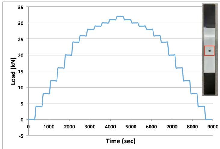
Figure 4.2: Load step plot for tensile testing of the OHT CFRP sample with paint-based PS coating. An image of the OHT CFRP sample is shown on the right with the mapped region boxed in red.
