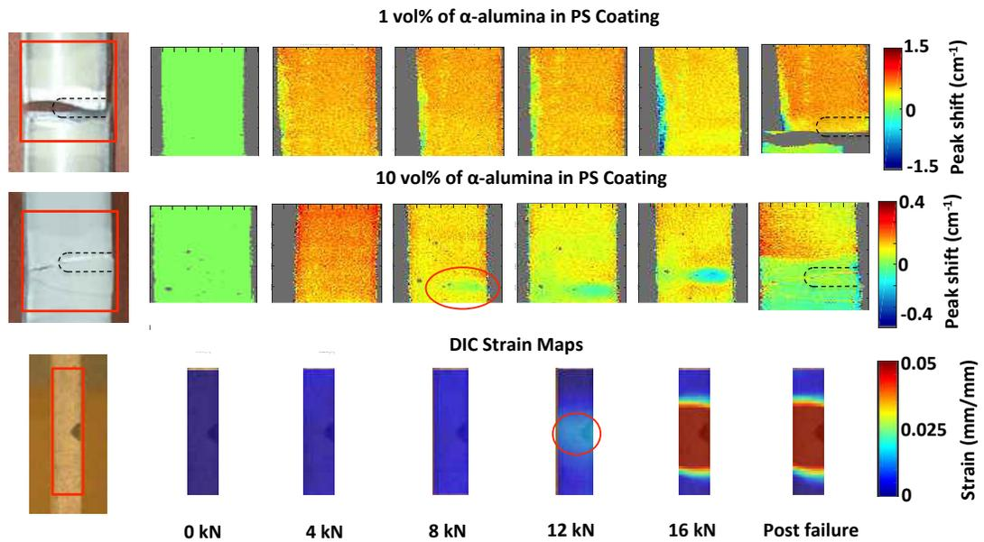
Figure 2.9: Images of the mapped regions of the samples are shown alongside the corresponding R1 peak shift maps (top and middle rows) and DIC strain maps (bottom row) with increasing load. Damage progression of the subsurface notch was detected by the PS coating with 10 vol% alumina at 8 kN before DIC detected damage progression at 12 kN. The PS map dimensions are 18 mm  $\times$  30 mm. DIC maps were taken from the center of the side of the sample, which was 4.826 mm in width.
