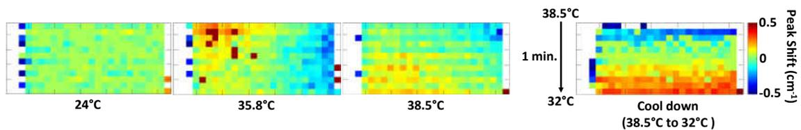
Figure 4.9: Peak shift maps showing changes in peak position with increasing (room temperature (24°C) to 38.5°C) and decreasing (38.5°C to 32°C) temperature from the unstressed state.
