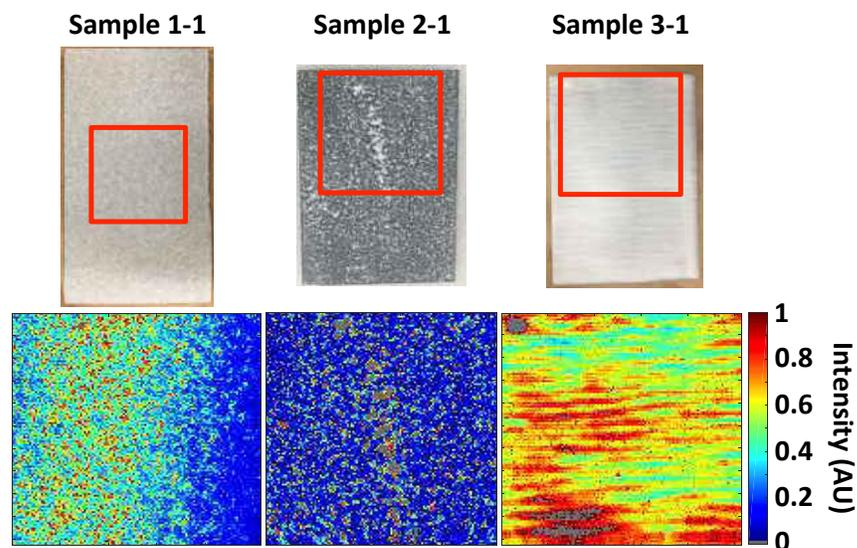
Figure 3.3: Representative samples (top row) with their corresponding normalized dispersion maps (bottom row) showing  $\alpha$ -alumina nanoparticle dispersion. Sample 1-1 was made using high shear mixing and spray gun. Sample 2-1 was made using high shear mixing and a paint roller. Sample 3-1 was made using planetary centrifugal mixing and a paint roller.
