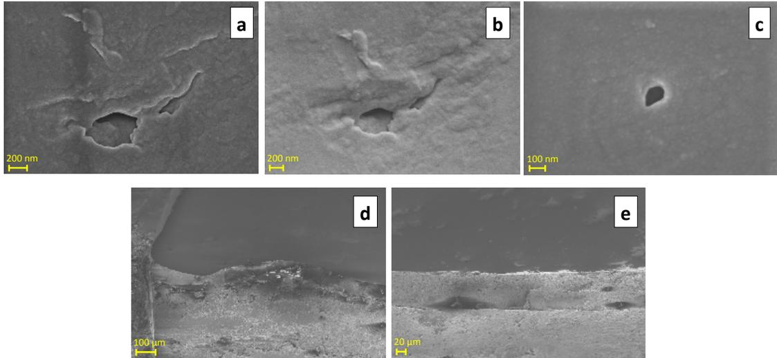
Figure 4.7: The SEM images shown here were taken from a sample with paint-based PS coating that was not subjected to load tests. Pores were found on the surface (a, b and c) as well as the cross section of the coating (d and e).
