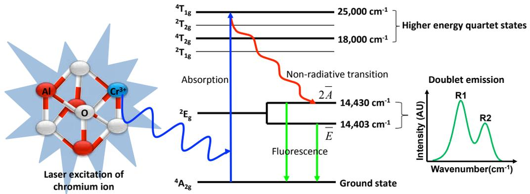
Figure 1.1: A schematic showing the emission of energy from chromium ions in  $\alpha$ -alumina resulting in R-lines.
