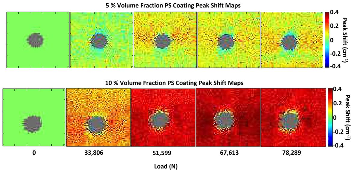
Figure 2.3: Stress sensing of two OHT CFRP specimens with 5 % and 10 % volume fraction PS coating with progressing loads. These specimens consist of composite substrates with hard laminate. Each map has dimensions of 25.4 mm  $\times$  25.4 mm.
