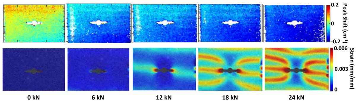
Figure 4.3: PS (top row) and DIC (bottom row) contour plots showing change in peak shift and strain, respectively, with increasing load. For the peak shift maps, the data points are with reference to their local zero load peak position.
