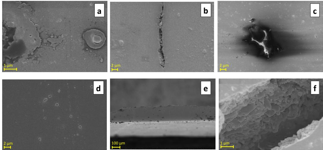
Figure 4.8: The SEM images taken after load tests indicate microcracks (a and b), agglomerations (c and d), pores (d) and uneven surface (e). The inside of one of the microcracks (f) reveals a granular structure within the paint-based PS coating.
