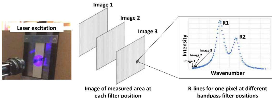
Figure 5.3: Schematic of data acquisition via laser excitation of the PS coating and image capture at each filter position.
