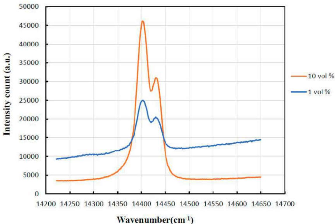
Figure 2.8: R-lines obtained from each sample at zero applied load.
