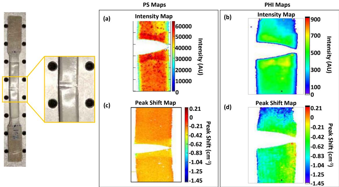
Figure 5.5: Close-up view of the mapped area on the aluminum tensile specimen with PS coating consisting of 10 vol%  $\alpha$ -alumina in PS coating with comparisons of dispersion maps from the (a) PS system and (b) PHI; and peak shift maps from the (c) PS system and (d) PHI system. Each map is 16.8 mm  $\times$  28.8 mm.
