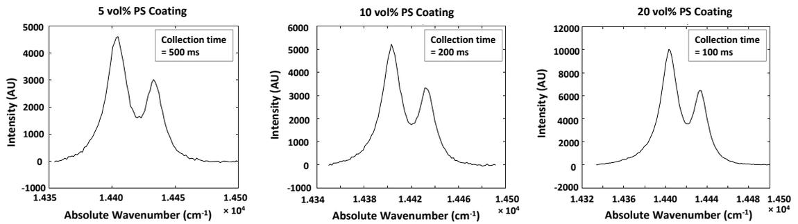
Figure 2.1: Representative R-lines for each PS coating with corresponding collection times.
