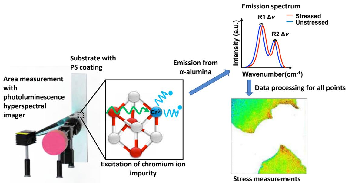
Figure 5.1: Targeted application for next generation stress sensing using the area measuring capability of the photoluminescence hyperspectral imager.
