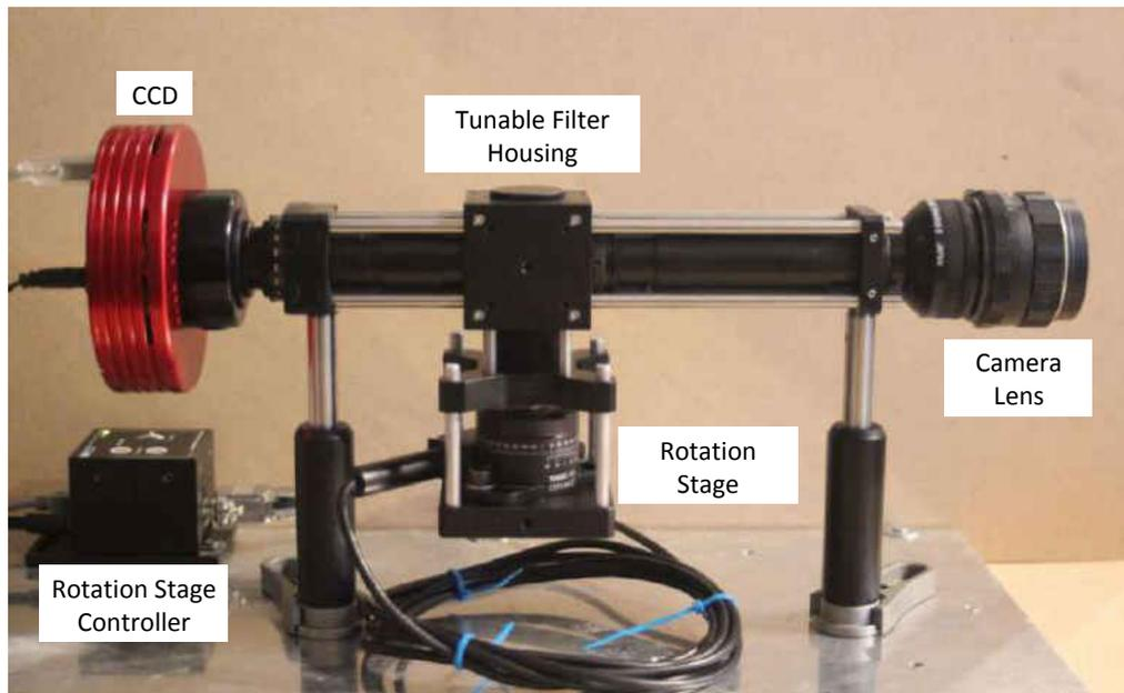
Figure 5.2: The photoluminescence hyperspectral imager and its major components.
