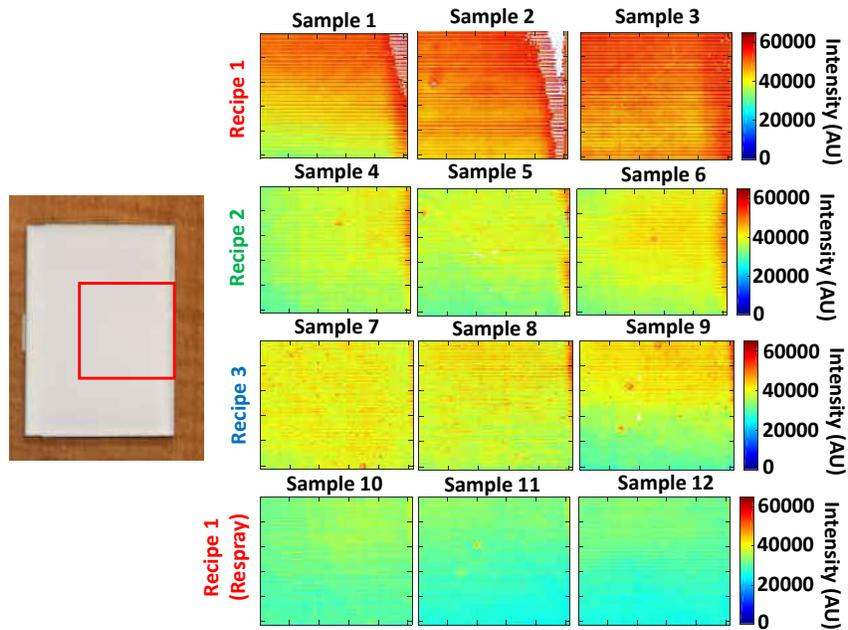
Figure 3.5: Comparison of paint-based PS coating particle dispersion via PL spectroscopy. The sample shown on the left is 101.6 mm  $\times$  76.2 mm.
