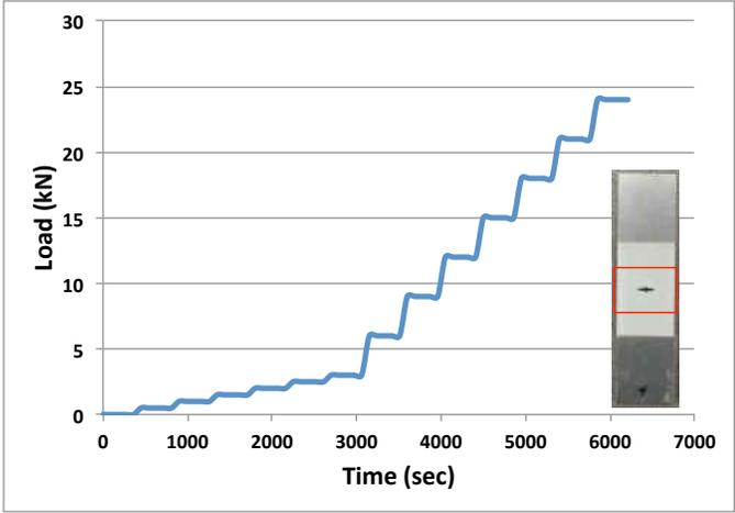
Figure 4.1: A load step plot for tensile testing of the notched Al-2024 sample with paint-based PS coating. An image of the notched Al-2024 sample is shown on the right with the mapped region boxed in red.
