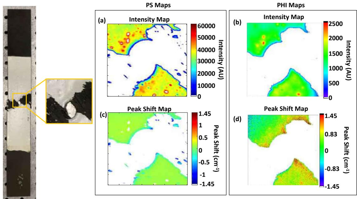
Figure 5.4: Close-up view of the mapped area on the OHT CFRP specimen with PS coating consisting of 20 vol%  $\alpha$ -alumina in PS coating with comparisons of dispersion maps from the (a) PS system and (b) PHI; and peak shift maps from the (c) PS system and (d) PHI system. Each map is 14 mm  $\times$  14 mm.
