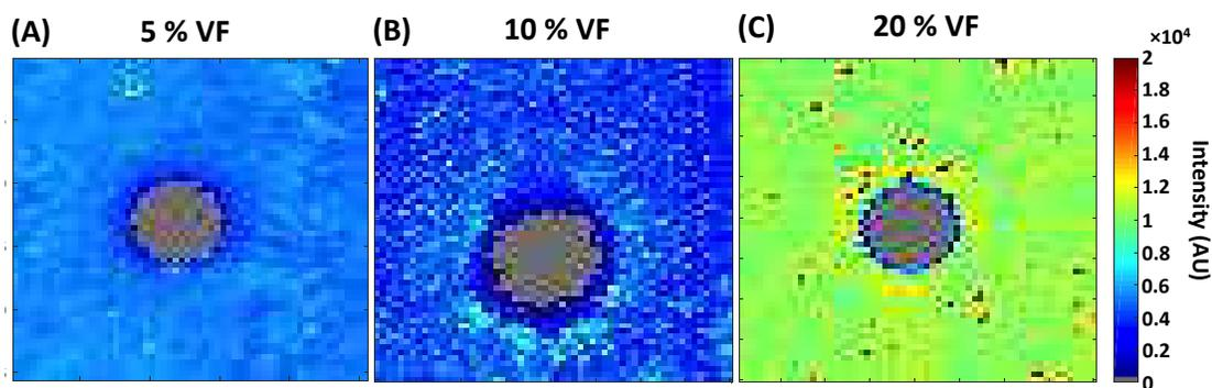
Figure 2.2: Contour maps showing  $\alpha$ -alumina nanoparticle dispersion for (A) 5 %, (B) 10 % and (C) 20 % volume fraction PS coatings. Each map has dimensions of 25.4 mm  $\times$  25.4 mm. Also, note that "VF" is volume fraction.
