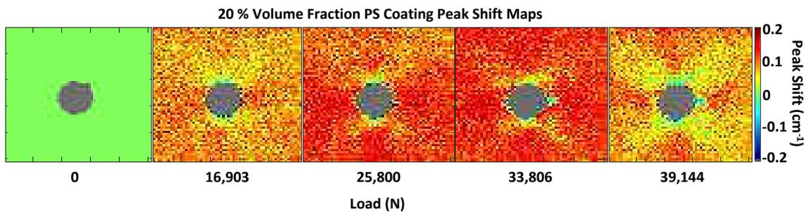
Figure 2.4: Stress sensing the OHT CFRP specimen 20 % volume fraction PS coating with progressing loads. This specimen consists of a composite substrate with soft laminate. Each map has dimensions of 25.4 mm  $\times$  25.4 mm.
