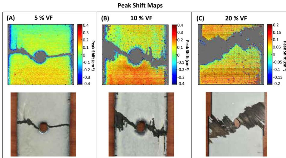
Figure 2.5: Contour maps with corresponding images of the OHT CFRP specimens showing peak shifts for (A) 5 %, (B) 10 % and (C) 20 % volume fraction PS coatings. Each map has dimensions of 40 mm × 40 mm. Also, note that "VF" is volume fraction.
