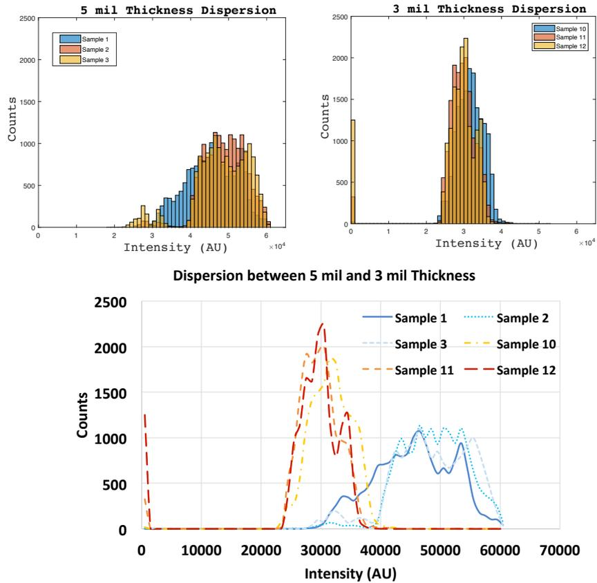
Figure 3.6: Histograms were plotted to show frequency distribution of intensities for different paint-based PS coating thicknesses. "Counts" pertain to the number of instances of an R1 intensity value.
