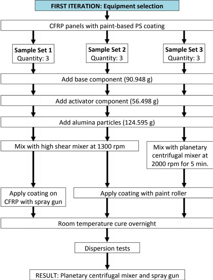
Figure 3.1: Flowchart showing the paint-based PS coating process approaches used in the first iteration. The selected equipment were implemented into the second iteration of coating manufacturing.
