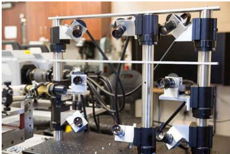
Figure 21: Image of the seeded air jet experiment, only corner imagers used to take data.
