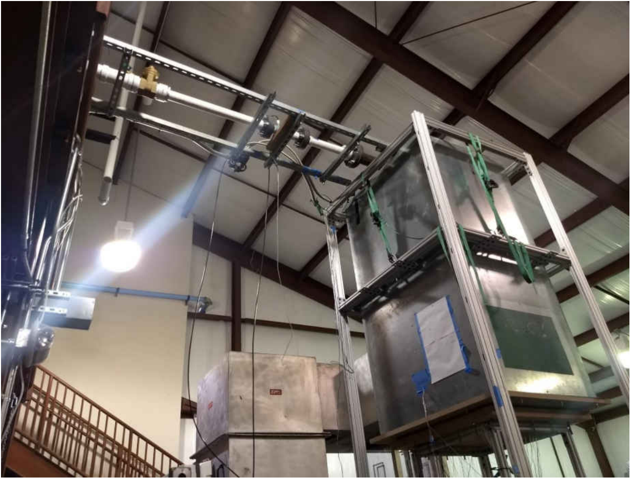
Figure 67: Experimental Plenum and Venturi
