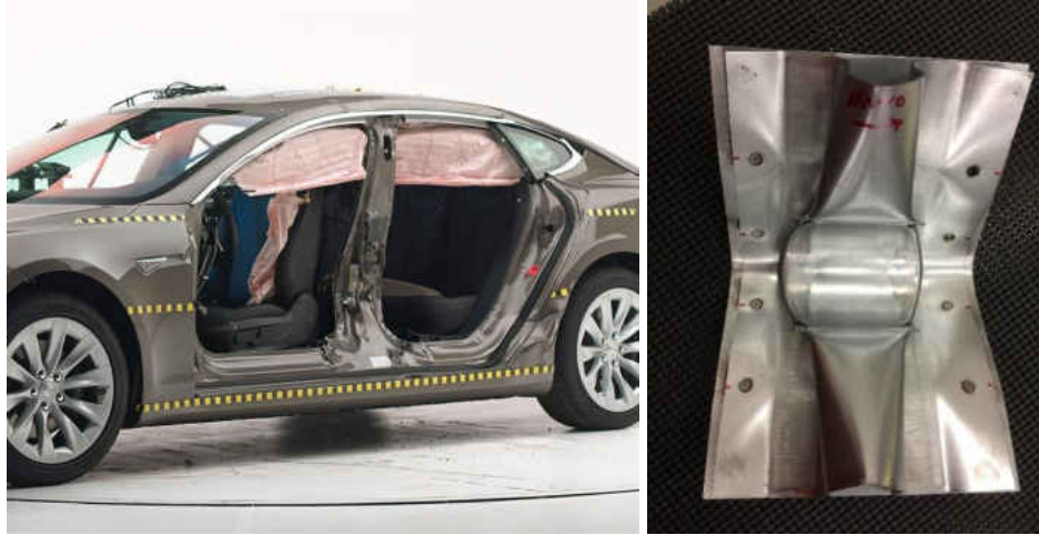
Figure 6-3. (a) B-pillar bending example (2016 Tesla Model S side IIHS crash test) (b) an example of three-point bending test on a hat section sample
