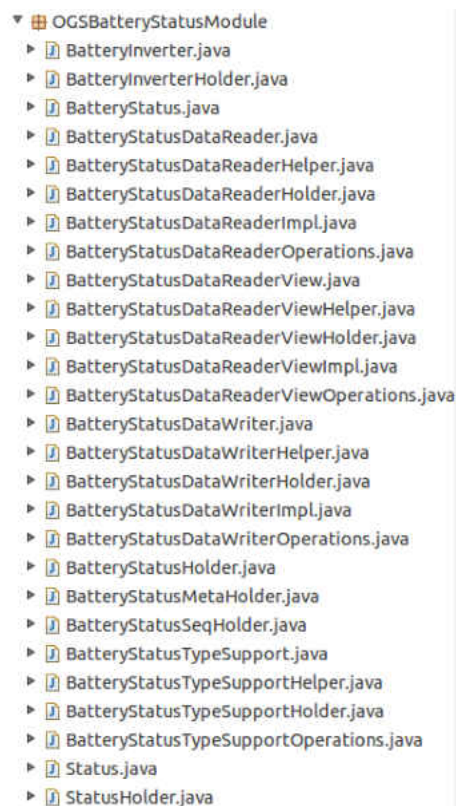
Figure 5-50: Screenshot of Java Classes Generated from the BatteryStatusModule IDL File
