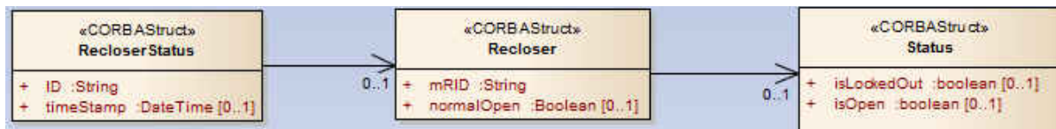
Figure 5-48: CIM-based UML Profile for RecloserStatus module
