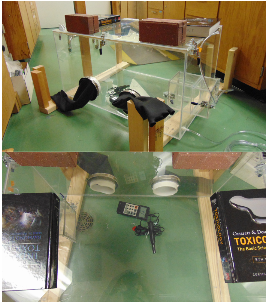
Figure A4. Completed Exposure Chamber – Oxygen Retention Testing. (Top) Upon completion of the acrylic exposure chamber (Top), measurements of internal oxygen concentration were made with respect to time, as presented in Figure 4 after reducing internal oxygen concentration to 5.4 % mol/mol with pure nitrogen. During testing, a handheld oximeter was utilized to monitor in real-time the oxygen concentration. (Bottom) The image shows the placement of the oximeter within the main chamber during measurements taken up to 99.5 hours after initial oxygen concentration reduction. At this time point, the internal oxygen concentration was 8.4 % at approximately 58 hour.
