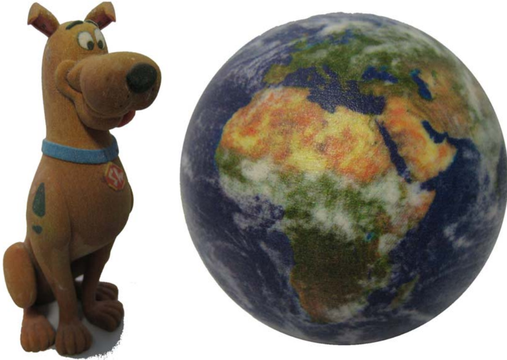
Figure 16. Examples of parts produced complete with color information.
