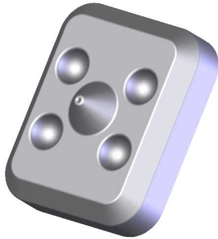
Figure 2. A solid model comprised of several solid geometric shapes merged through a Boolean operation.
