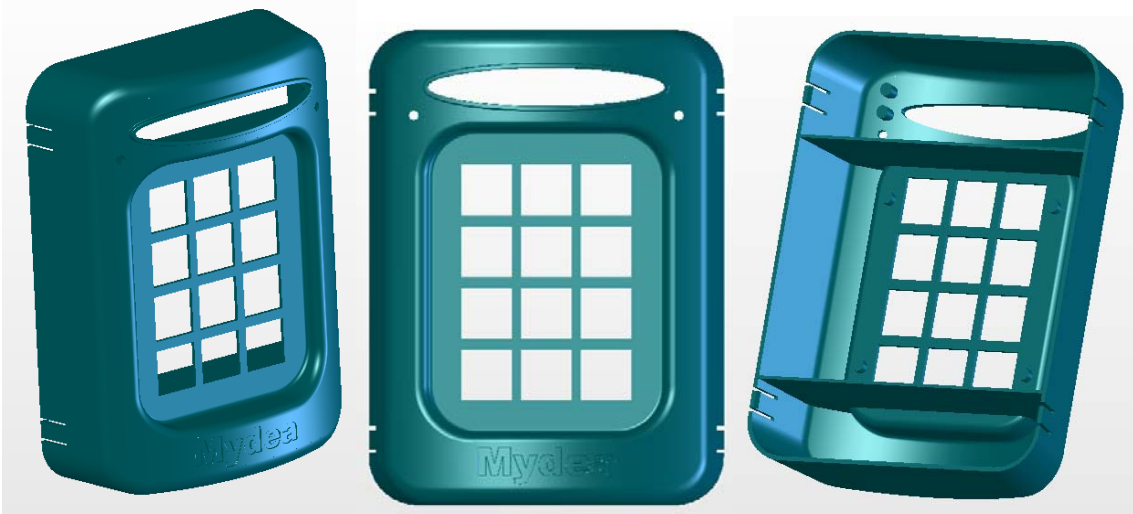
Figure 28. The electrical component housing used in the case study.
