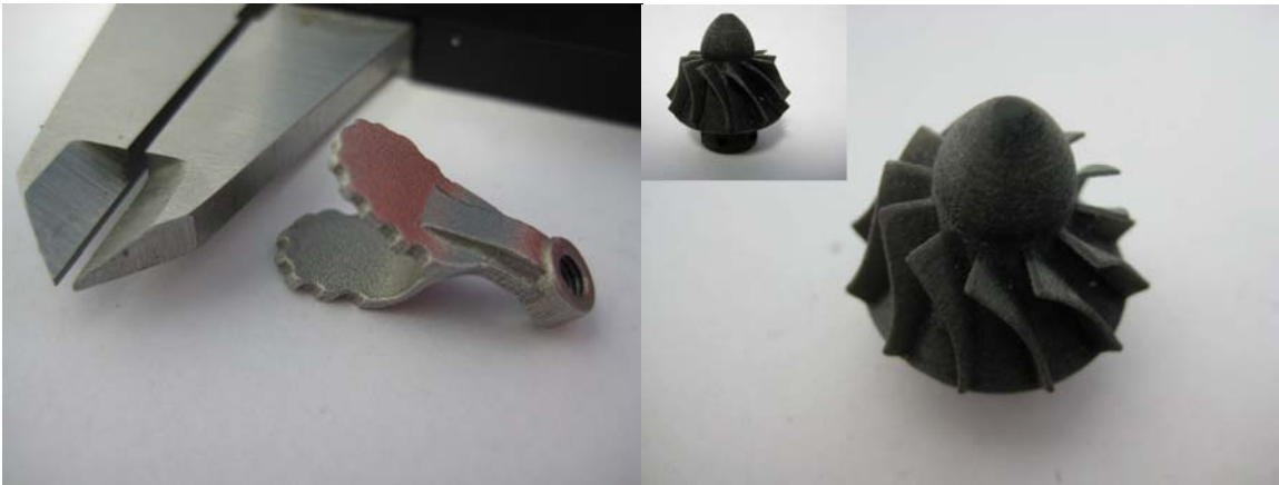
Figure 19. Examples of parts with features that may be considered 'small' for common AF technologies.
