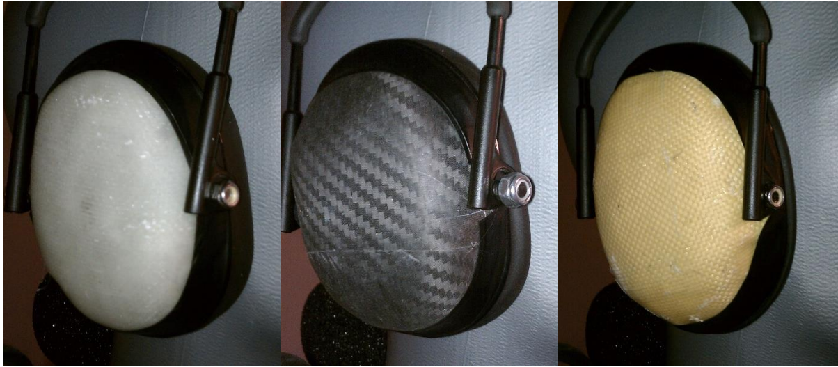
Figure 11 - 3M FRPC Ear Cups (left to right: Glass, Carbon, Aramid)
