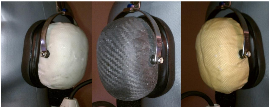
Figure 9 - FDC FRPC Ear Cups (left to right: Glass, Carbon, Aramid)
