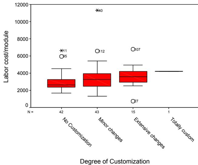
Figure 21- Box Plot for Labor\$/Module of HUD-Code Plants
