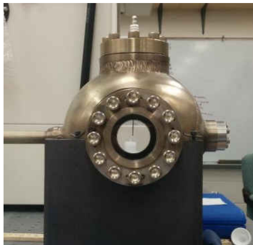
Figure A1. Side view of the spherical combustion chamber with a regular spark ignition system.
