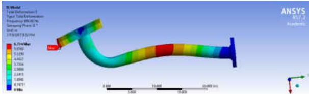
Figure 40 The 5th Mode for FPA, 2 Inch Diameter, CS, 24 Inches Long
