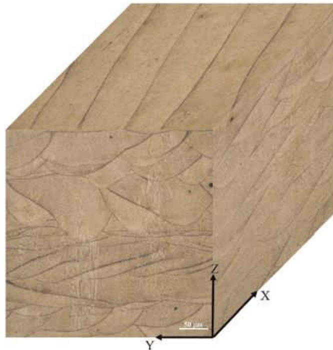
Figure 2.3 - Cross-sectioned SLM sample displaying typical macrostructural features [81].
