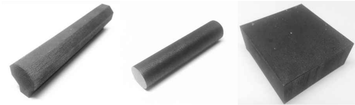
Figure 3.2 - Hexagonal transverse and round longitudinal bars produced for full-sized tension samples and blocks produced for fracture tests, all of which were utilized for SPT samples.
