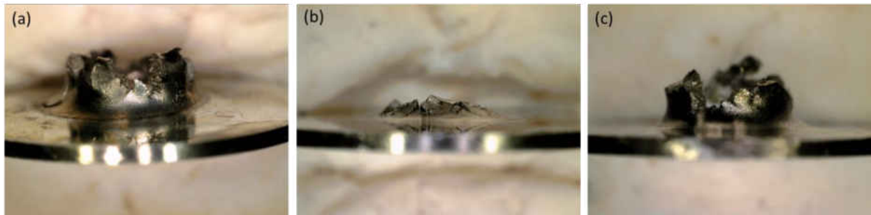
Figure 5.39 - Fracture of cyclically loaded 304SS samples at 200°C with control modes of (a) R=-1 load control, (b) R=-1 displacement control, and (c) R=-1 load control with 15s hold time.
