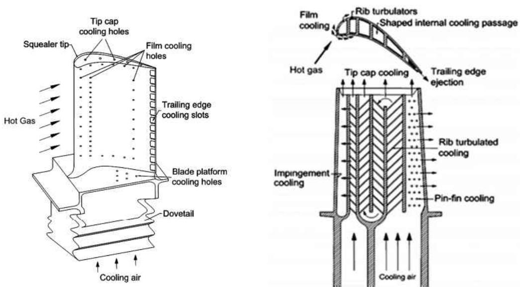
Figure 2 Schematic of turbine airfoil with different cooling technologies in different zones [1]
