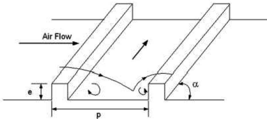
Figure 3 Flow separation by angled ribs [1]
