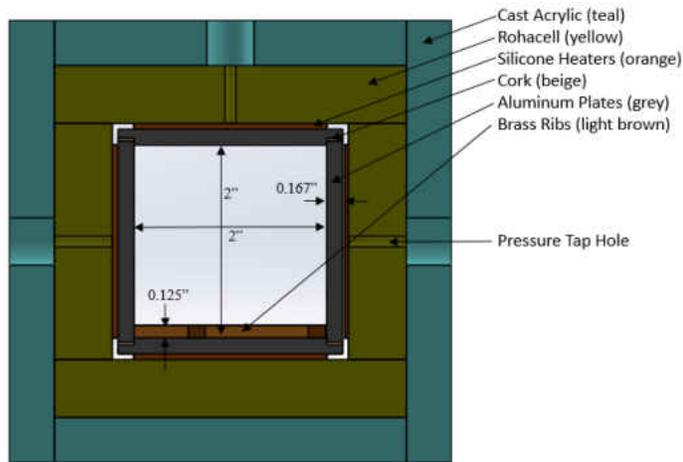
Figure 5 Cross-sectional view of the one ribbed wall case
