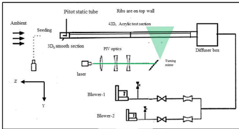
Figure 10 Schematic of the PIV rig set up
