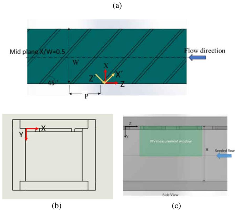
The coordinate system for the PIV tests is shown in Figure 9. Stereoscopic (2D-3C) PIV was used for the investigation. Stereo PIV can determine all the three velocity components as well as all the six Reynolds stresses. Table 7 shows the test matrix of the PIV tests.
