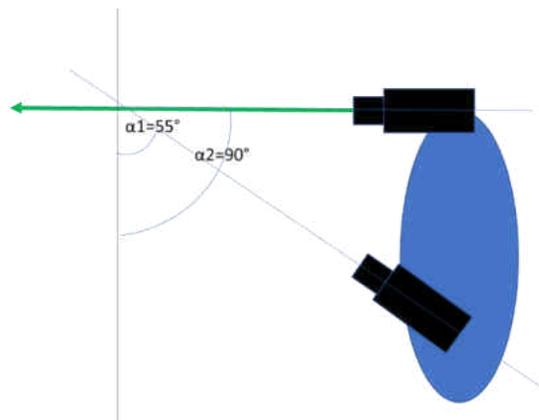
Figure 75 Asymmetric camera arrangement for the current study
