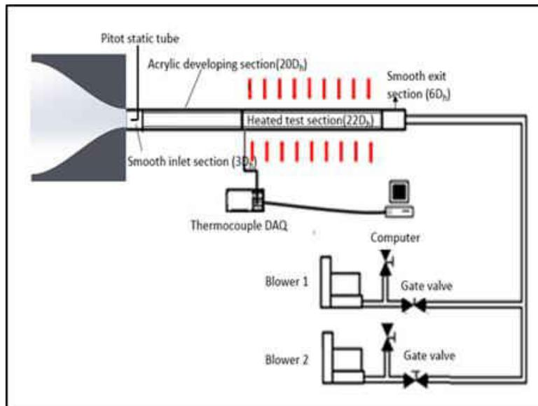
Figure 6 Experimental layout for heat transfer test
