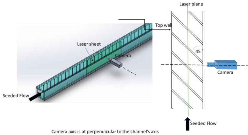
Figure 88 2D planer PIV measurement set up
