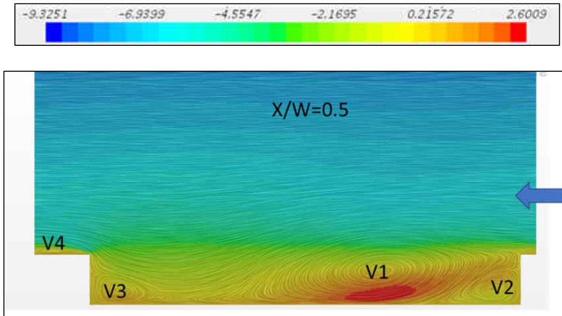
Figure 34 LES results of mean velocity  $V_z'$  in the streamwise midplane at  $Re \approx 30k$
