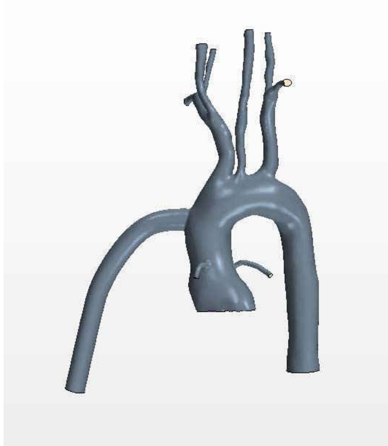
Figure 25 - Sample of patient specific geometry obtained from CT scans with LVAD cannula anastomosed to the ascending aorta.
