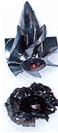
Thrombus formation around the impeller of an exchanged MicroMed DeBakey VAD.
