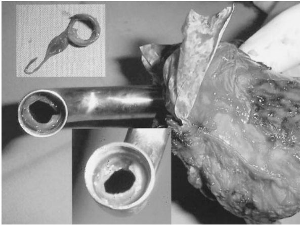
Thrombus formation in the inflow conduit of a MicroMed DeBakey VAD.
