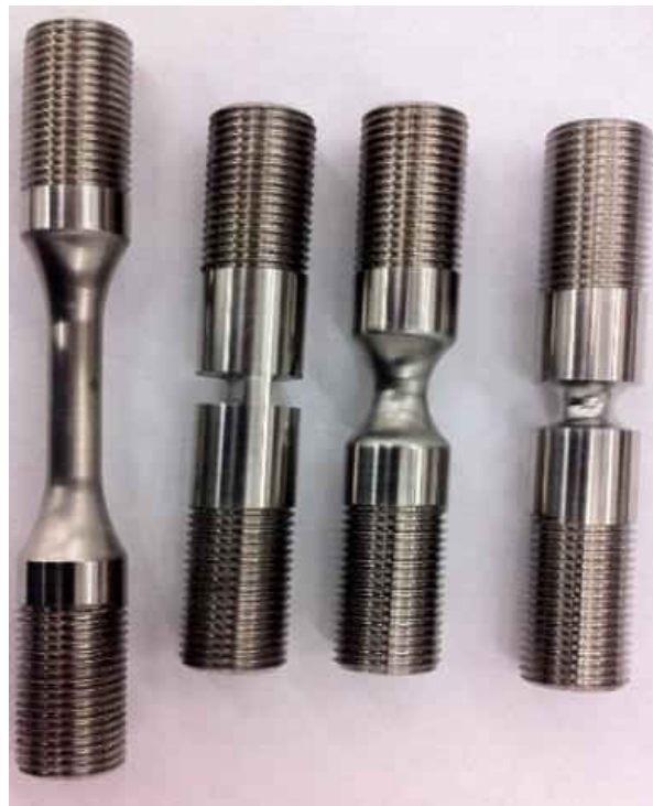
Figure 27: Real specimens before testing denoted as R0, PE, R2, and R1 from left to right.
