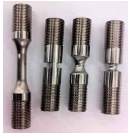
Figure 17: (a) Symbol notation of the cross section of a notched specimen (b) Four different shapes of the specimens before fracture.
