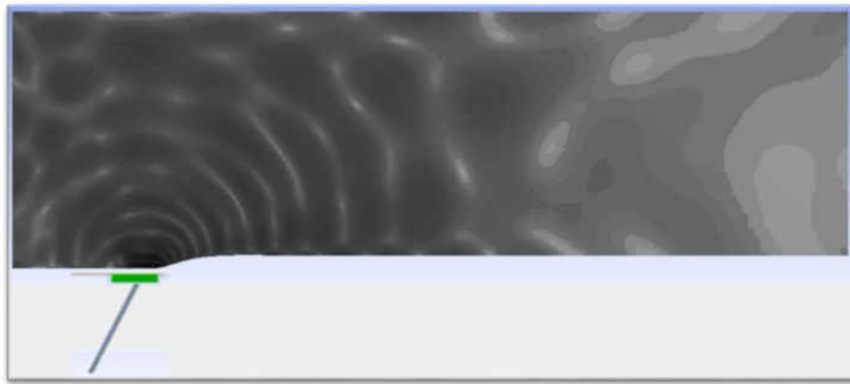
Figure 4-7 Stress distribution through the tissue layer at the fully-closed position where the top leaflet hits the valve housing.
