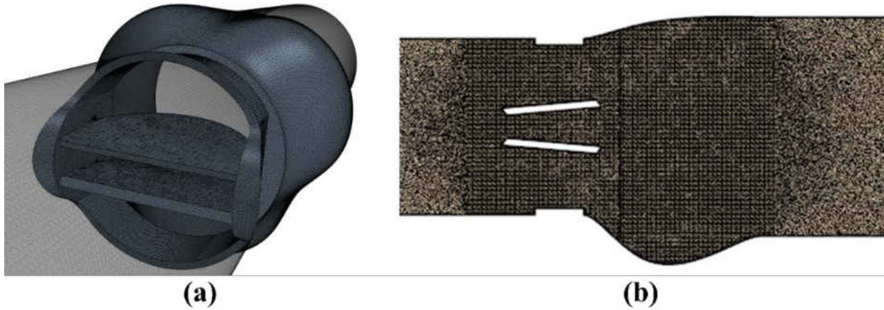
Figure 3-9 High quality polyhedral mesh generated (a) close to the wall and leaflet surfaces and, (b) in the flow domain.
