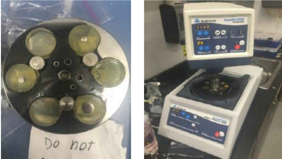
Figure 3-5: Mounted specimens (a) and Buehler EcoMet3000 polisher (b).
