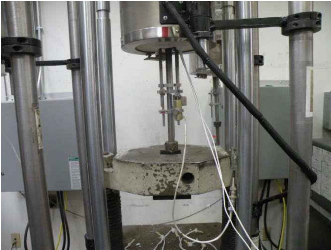
Figure 3-2: Experimental set-up for tensile testing.
