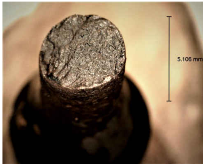
Figure A- 13. Pictures of deformed specimen BR15.
