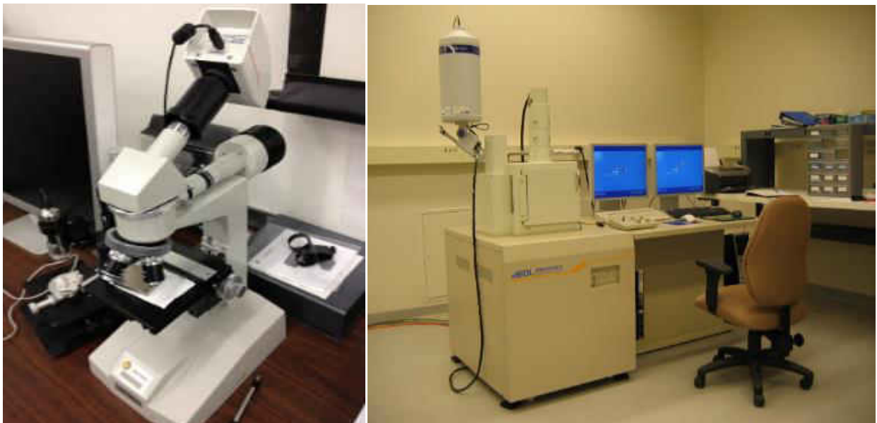
Figure 3-6: Microscopy equipment, a) Excel Tech MEF3 Microscope and b) Scanning Electron Microscope.
