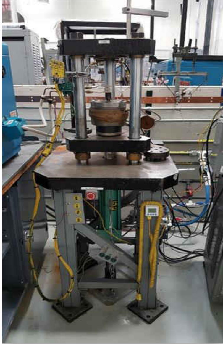
Figure 3-3: Experimental set-up for fatigue testing.
