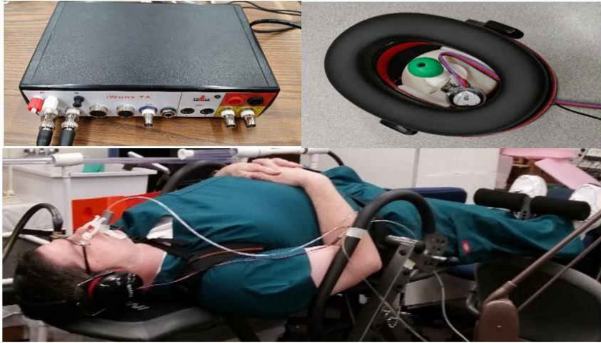
Figure 3-1 Experimental setup showing: the data acquisition system, the Piezo sensor assembly, and spirometer assembly (top row). The bottom picture shows the subject wearing piezo sensor headset while the spirometer is put into subject's mouth to acquire the breathing data.
