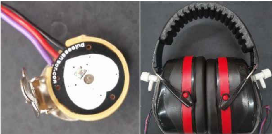
Figure 2-2 (a) Ear lobe pulse sensor (b) TMp sensor assembly. The piezo sensors and the ear lobe sensors are inside the right and left ear muffs. The while valves are used to test air tightness between ear canal and piezo disc by connecting the valve outlet to a manometer
