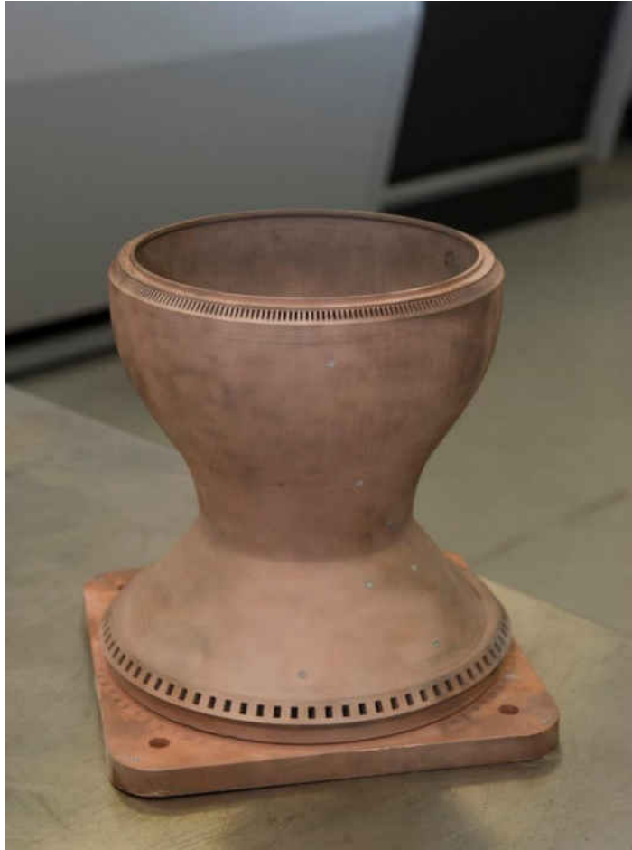
Figure 10: Additively Manufactured Copper Thrust Chamber [11]
