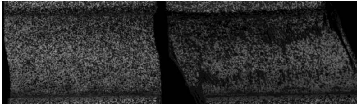
Figure 12: Comparison of last test step in shear tests between displacement control (left) and force control (right) shear tests
