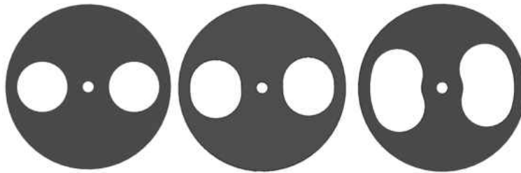
Figure 3.11: DC Disks: 27% (left), 33%(center), and 50% (right)
