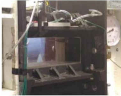
Figure 3-6: Test Section Addition for Pressure Sensor and Transducer Instrumentation
