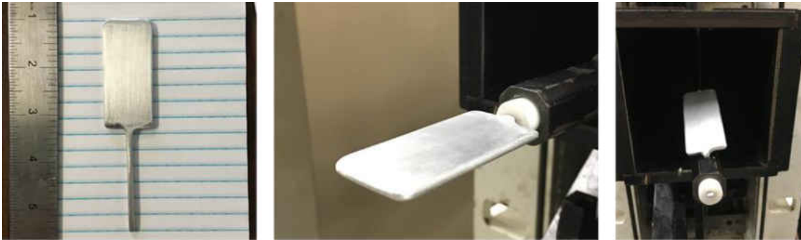
Figure 2-18: Test Electrode Wind Tunnel Test
