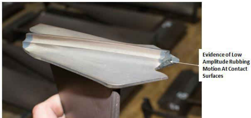
Figure 43: Contact surface condition after removal from engine
