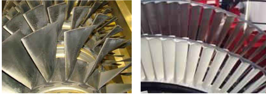
Figure 1: a) Cantilevered compressor blades b) Shrouded turbine blades
