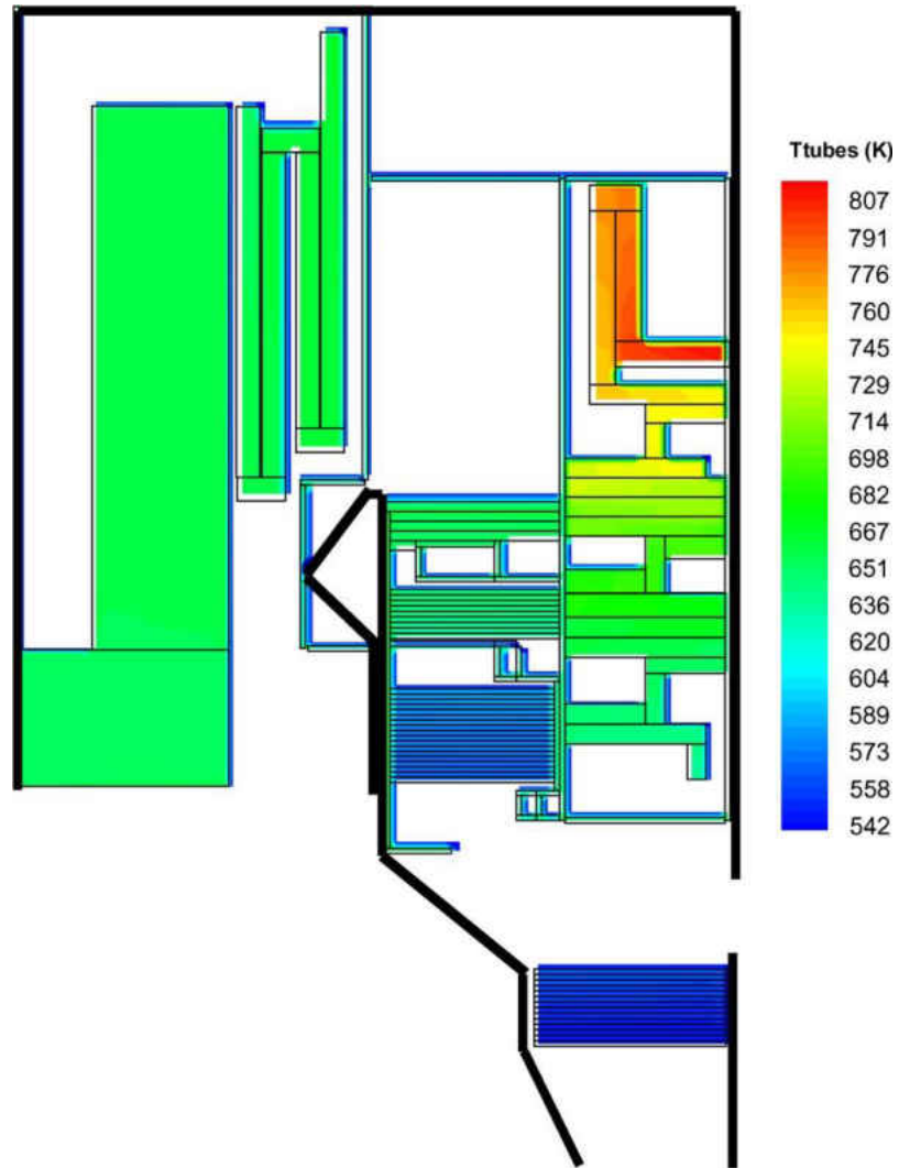
Figure 31) CFD simulation of temperature distribution in the convection zone of a power boiler
