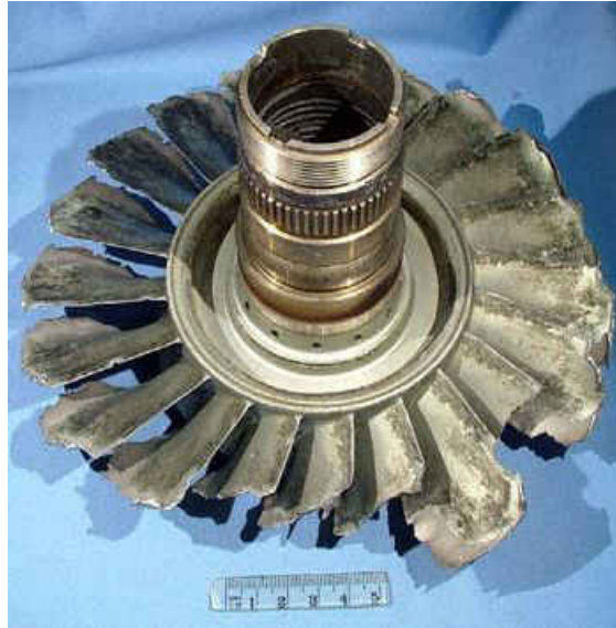
Figure 1.1: Example of Blade Failure. From ATSB
