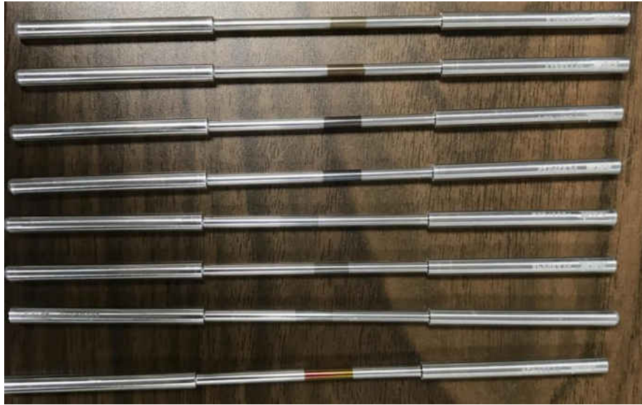
Figure 30: Reference tubes with theoretically known deposit thicknesses
