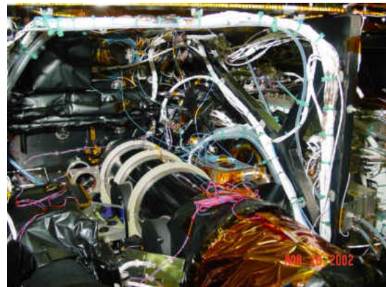
(b) Data cabling attached to various tie-down points.
