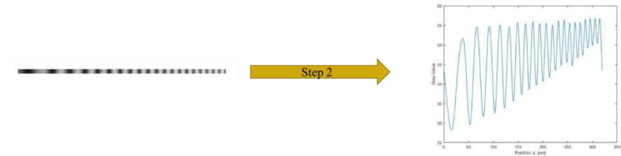
Figure 13: Step 2, (Left) Selected region of interest of gray value image, (Right) Plot of the gray values as a function of position ( x ).
