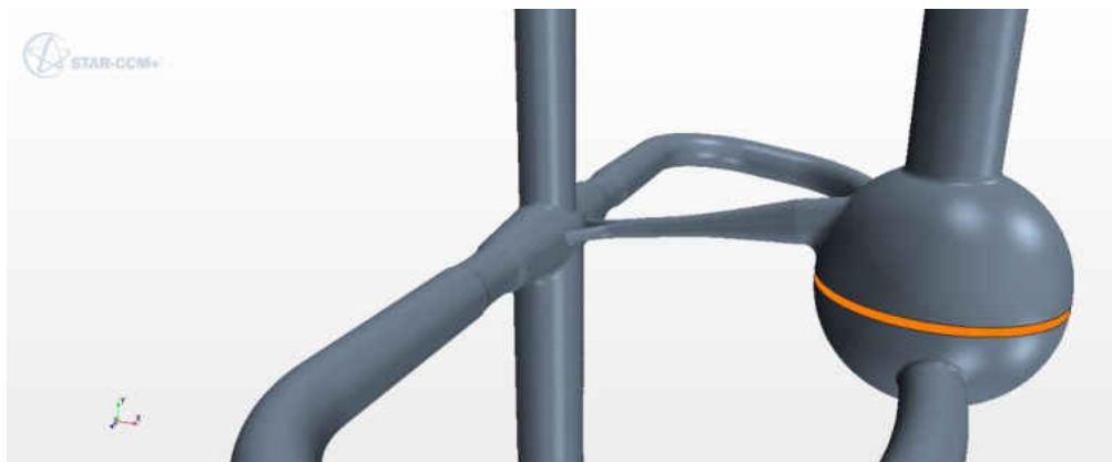
Figure 44: Venturi Effect by Reducing Pulmonary Artery Flow Area.
