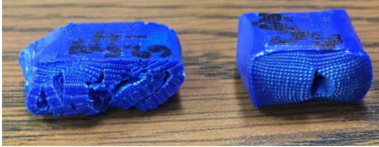
Figure 4.29: Comparison of Z+67.5 (left) and Z+45 (right) specimens after compressive testing
