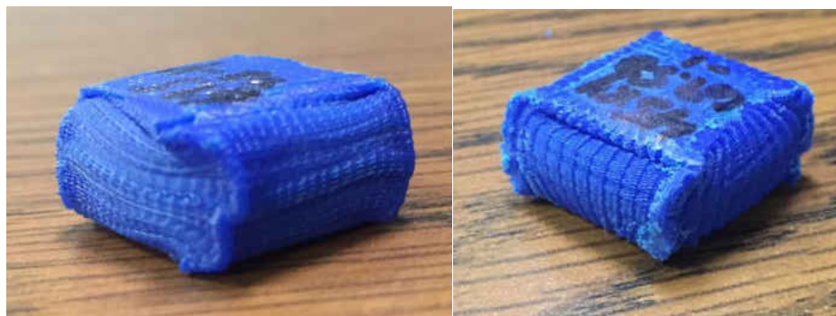
Figure 4.31: The Y-67.5 (left) and Y-67.5/Z+45 (right) specimens after testing.
