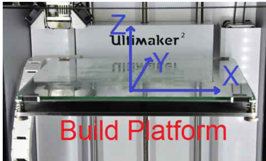
Figure 3.4: Illustration of the coordinate system of the printer
