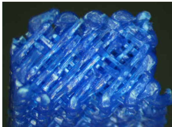
Figure 4.17: Failure surface for Y-45/Z+45 orientation
