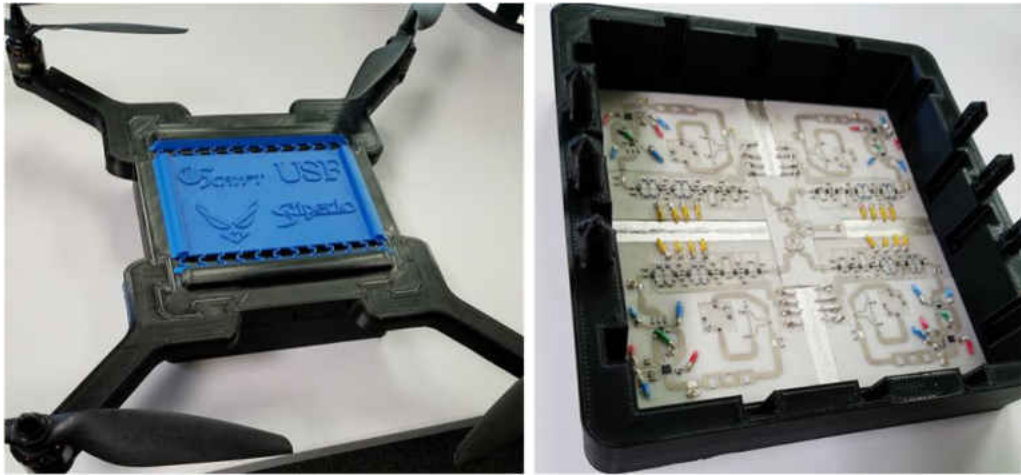
Figure 1.1: 3D printed quadcopter (left) with internal fully printed complex RF electronics (right) [1]
