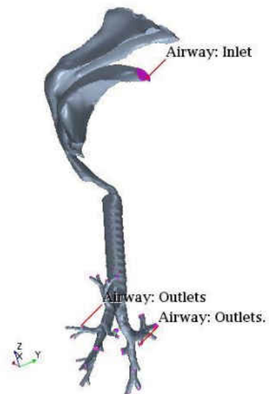
Figure 5-3: Airway CFD boundary conditions
